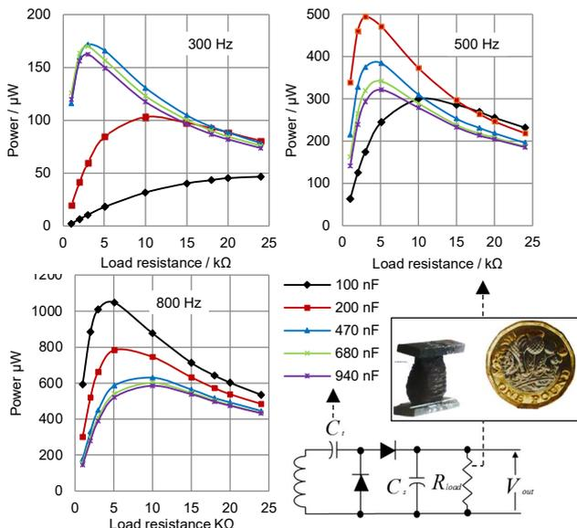
Fig. 7: Measurements from the Schottky voltage doubler circuit (bottom right) demonstrating harvesting power in the 0.1 – 1 mW range, reactance elimination by tuning  $C_i$  and load matching for three different frequencies. A photograph of the 1:7 funnelling device is also shown.
