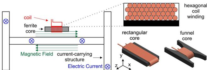
Fig. 1. The concept of inductive harvesting from a current-carrying structure. Coil winding and core shapes are illustrated on the right.
