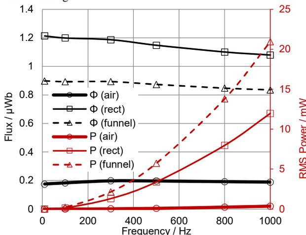
Fig. 5: Simulated flux and power output from a  $40 \times 5$  mm frame without a core, with a rectangular core and with a funnel-shaped core at its  $10 \times 5$  mm neck frame. For the power output calculations, a 2500 turns, hexagonally packed 0.04 mm Cu wire coil is assumed. The structural current amplitude is 200 A.
