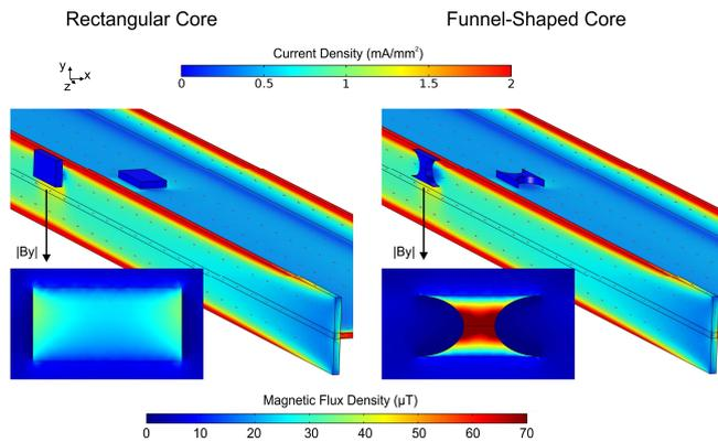
Fig. 4: Simulated current and flux density for two magnetic soft-core geometries, for a 1 A, 1 kHz total structure current.
