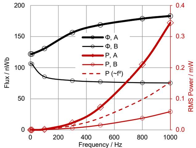
Fig. 3: Simulated flux and power from a  $40 \times 5$  mm frame at locations A and B in Fig. 2, with a 2500 turn, 0.04 mm Cu wire, from a 200 A current.
