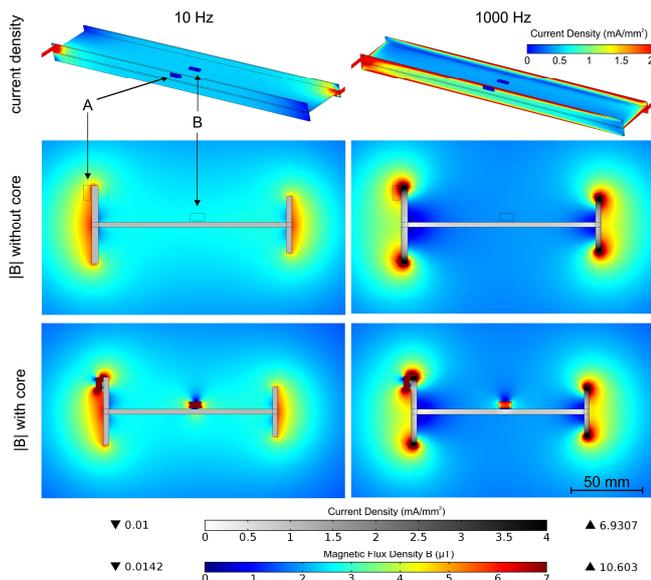
Fig. 2: Comsol simulation of current density J and magnetic flux density B in a structural beam, for 10 Hz (Left) and 1 kHz (Right), 1 A current.
