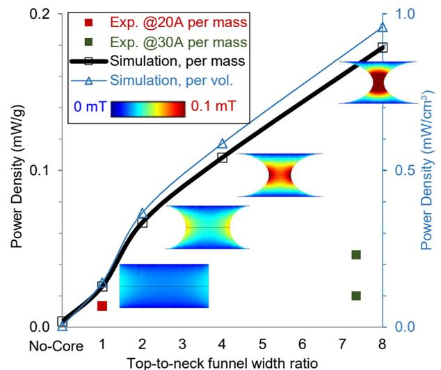
Fig. 6: Calculated power output density as a function of funnel core narrowing ratio, with 2500 turns of a 0.04 mm Cu wire hexagonally distributed around the core neck, for a 300 Hz, 200 A structural current. The flux density distributions are also shown, for a 1 A structural current.
