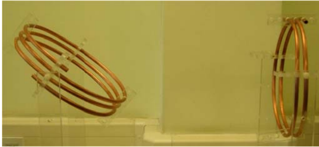
Figure 5 Misaligned 3 turn (left) and 2 turn (right) 30 cm diameter coils.
