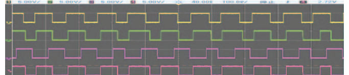
Fig. 7. Output bit streams from the four channels showing the recovered data rates at 10.3 bps.
