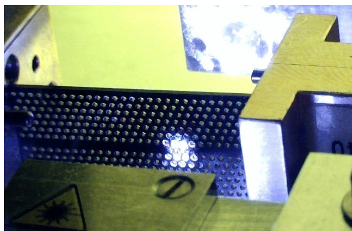
Fig. 4: Laser illumination spot on one side of the photonic crystal (as seen through an infrared/optical camera)
