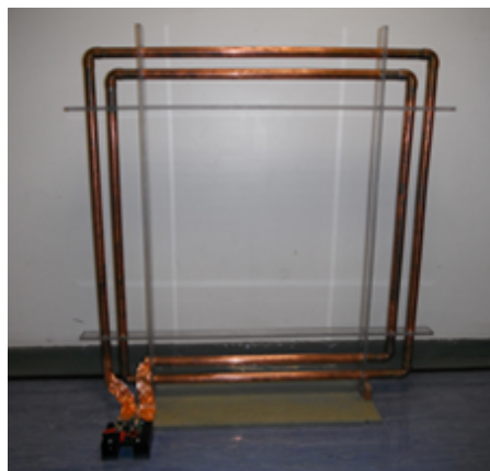
Figure 3. 1 m Tx coil and class-E amplifier
