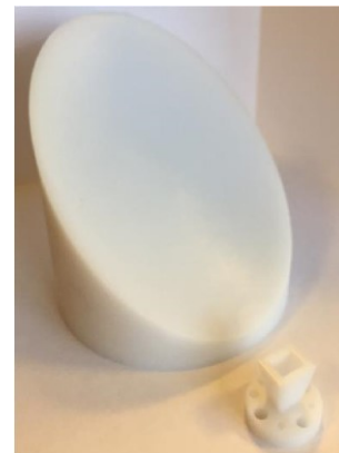
Fig. 4. Polyjet 3D printed rectangular horn antenna and parabolic mirror (prior to metal plating).
