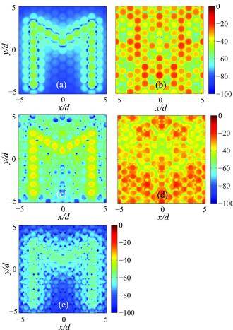
FIG. 11. (Color online) Near field imaging with a bilayered planar structure. Magnetic field distribution at five frequencies  $f_0$ =30, 40, 49.3, 55.7, and 65 MHz (a)-(e). The distance between the object and image plane is 15 mm.
