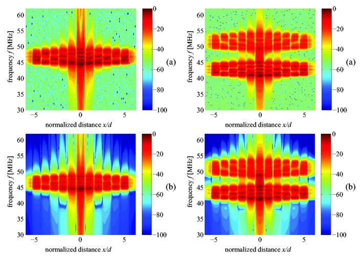
FIG. 4. (Color online) Near field imaging for the double lens with h =20 mm. Magnetic field distribution in the image plane vs frequency (contour plot). Experiment (a) and theory (b).
