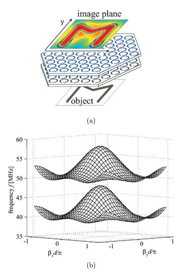
FIG. 10. (Color online) Bilayered magnetoinductive lens with hexagonally arranged elements. (a) The setup. (b) Dispersion surfaces  $f(\beta_x, \beta_y)$  of magnetoinductive waves supported by the structure (nearest neighbor interactions, no losses).
