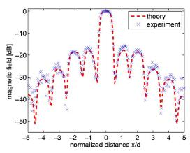
FIG. 6. (Color online) Theoretical (red curve) and experimental (blue crosses) magnetic field distribution in the image plane along the x axis for the double lens with h=10 mm separation at the resonant frequency (46.2)
