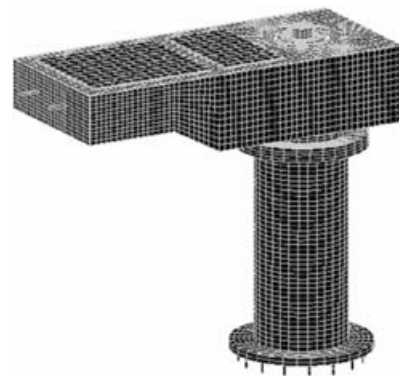
Fig. 5 FE model of the prepolariser support structure
