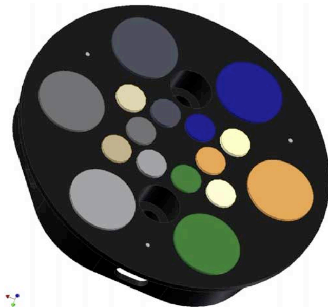
Figure 2. The ISWEEP magnet experiment and radiometric calibration target for the SSI. Six sweep magnets are built into an aluminum structure and covered with six different colors. The three small white spots are 0.75 mm in diameter and serves as internal fiducial points for the ISWEEP experiment. The black anodized housing is 52 mm in diameter.
