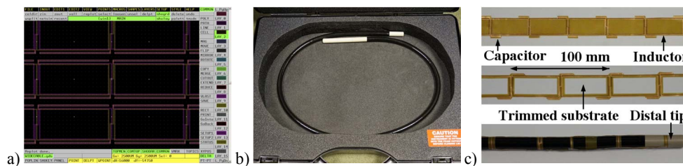
Fig. 4. a) CAD layout of PCBs; b) flexible insertion tube; c) PCB after frequency tuning, cutout and mounting. Non-magnetic insertion tubes with the design of Fig. 1b and a diameter of 13 mm were fabricated by the UK
