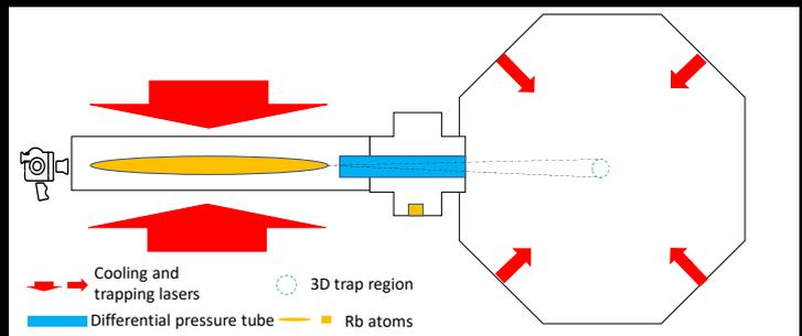
Figure 4 : Schematic diagram of experimental setup to produce 2D MOT and 3D MOT.
