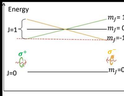
Figure 5 : Principle of Magneto Optical Trap and experimental results. The photon carrying opposite spinning direction counter-propagates in the presence of magnetic field. This lead to a trapping potential to capture atoms that will be used to perform atom interferometry.
