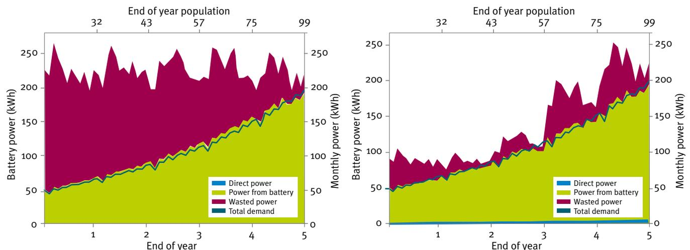
**Figure 2:** Monthly energy usage profiles for minigrad systems with connections increasing from 25 to 100 households over a five-year period. Both systems provide a minimum 95% reliability. **Left:** A static system designed to meet the demand of the final community size. **Right:** A modular system which is reassessed and resized if necessary every year to meet the growing demand.
