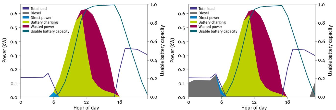
**Figure 1:** Average generated power usage by hour of the day. **Left:** Basic solar and battery system with 70% reliability. **Right:** The same solar and battery system with an additional diesel backup to achieve > 95% reliability.
