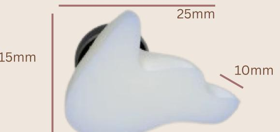
This is our model of NZ buds. The design ensures contact with the auricular branch of the vagus nerve while housing an electrode module and sensor without protruding from the ear.
