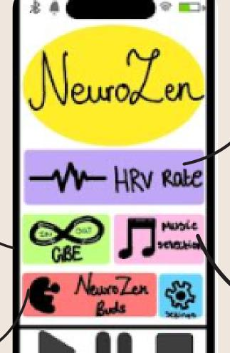
The app tracks heart rate variability (HRV), a key biomarker of vagus nerve function and autonomic nervous system activity. If HRV drops, the user receives a notification and the NZ buds deliver electrical signals. Over time, the app builds a personalized HRV profile, enabling users to monitor progress and adjust stimulation intensity. This is especially important
