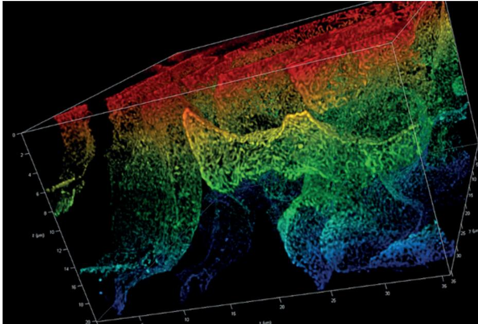
Nephrin in cleared kidney section. 3D STED at a depth of 130 to 150  $\mu\text{m}$  into the tissue, using the STED WHITE 93x glycerol objective lens. Immunostaining performed with Atto594. Sample courtesy of David Unnersjö Jess, KTH, Stockholm, Sweden.
