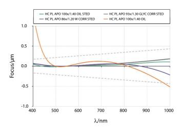
Figure 1. STED WHITE Class objective lenses: Chromatic correction over the  $400-1000\,\mathrm{nm}$  wavelength range.
