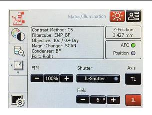
To Adjust the Brightfield use the microscope tab, open the brightfield (IL) shutter, and adjust intensity and condenser aperture, using the controls on the left side of the microscope stand
