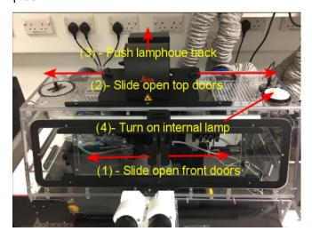
The chamber light can also be controlled with a footswitch once turned on
