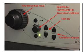
There are controls on the left-hand side of the microscope stand to control:
