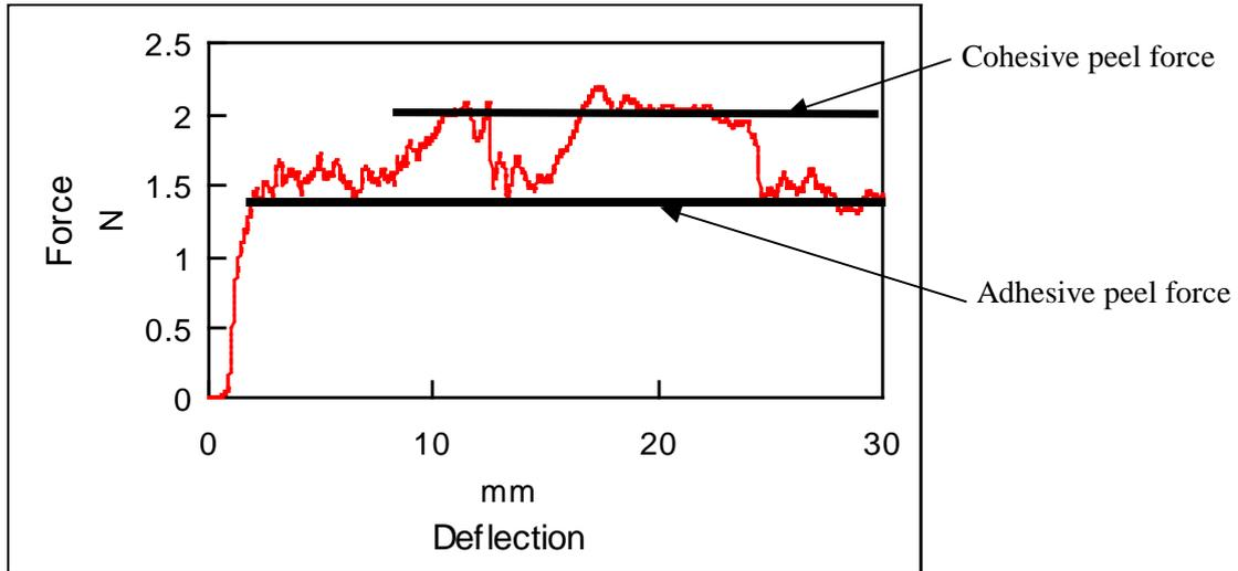
**Figure 6B Peel force versus deflection in a fixed arm peel test. The higher peel forces relate to cohesive fracture; the lower peel forces relate to adhesive fracture**
