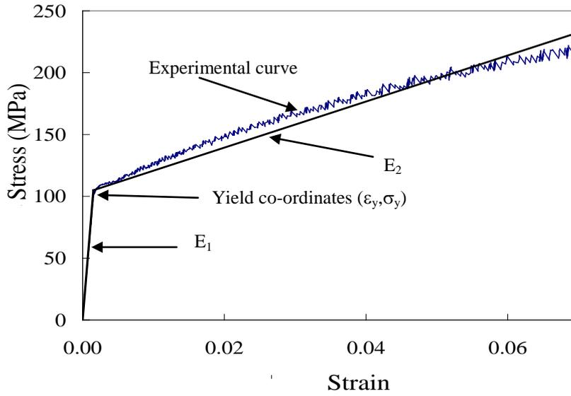
**Figure 3 Tensile stress versus strain plot for a peel arm illustrating a bilinear elastic-plastic fit and the definition of  $E_1$ ,  $E_2$  and yield strain**
