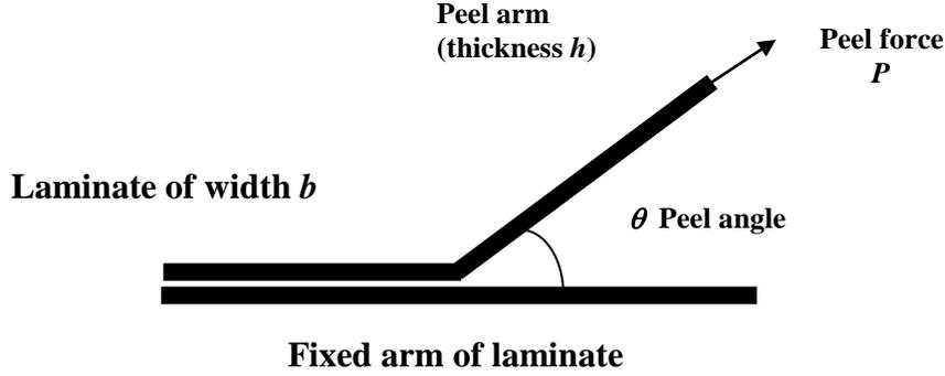
**Figure 1 Fixed arm peel test**
