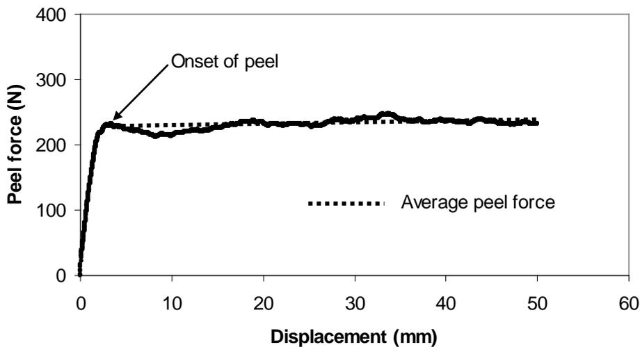
**Figure 6A: Illustrative peel force versus displacement demonstrating how to average the peel force.**
