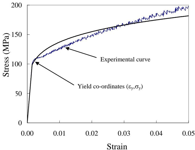
**Figure 4 An illustration of an elastic region followed by a power law fit for work hardening.**
