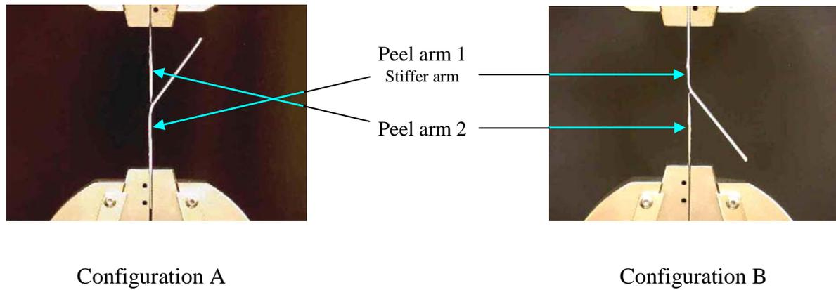
**Figure 8 Specimen configurations for T-peel**
