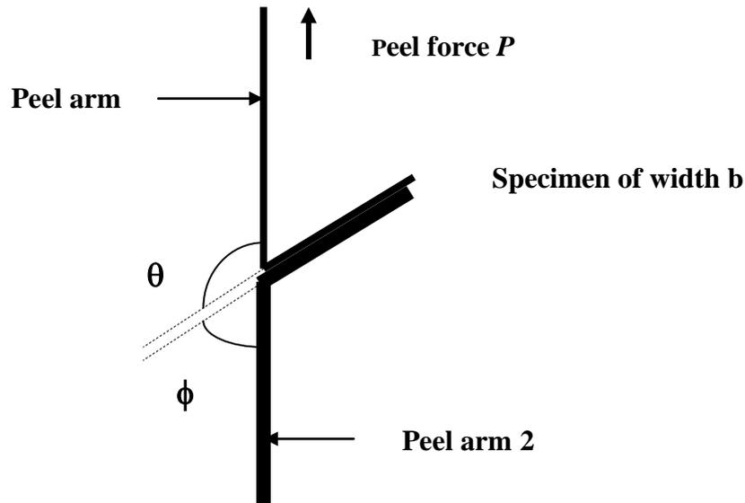
**Figure 7: T-Peel Specimen During a Test.**
