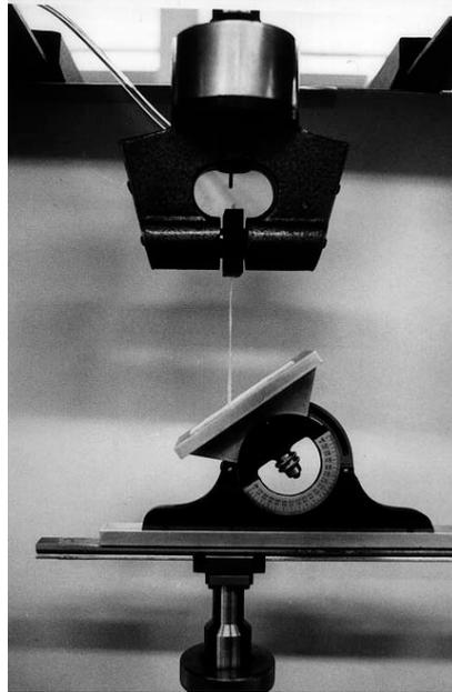
**Figure 5 Fixed arm peel fixture with linear bearing system showing a peel angle of 45°.**
