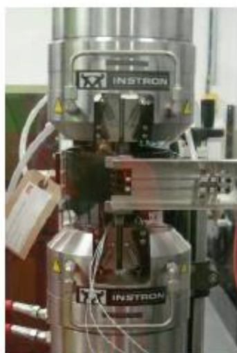
Induction-heated thermo-mechanical test rig
