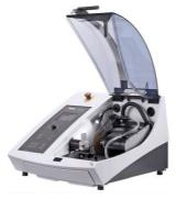
The CASC purchased, with the help of the department, an Accutom 100 from Struers. This saw is capable of cutting hard using diamond coated bladed but also to do programmable cuts. This allows the preparation of specimen with precisely controlled and repeatable sizes, for preparing specimen for mechanical testing for instance. In addition, this machine is capable of accurately grind and flatten the surface of samples using a diamond coated cup wheel, producing flat and parallel surfaces.
