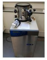
Freeze-drying is a drying process, where the solvent (normally water) is eliminated from the sample via direct sublimation from solid to gas phase. This is a useful way of eliminating solvents by keeping the material structure intact for further processing, like for example sintering.
