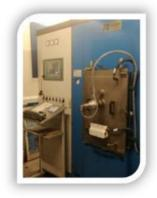
The vacuum hot press from FCT Systems is fully operational. The press operates at temperatures up to 2400oC for
