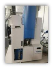
An Oxygen-Nitrogen-Hydrogen Elemental Mass Gas Analyser (Horiba, EMGA – 830 series) was installed at CASC in 2015. This includes also the Carbon-Sulphur Elemental Mass Induction Analyser (EMIA series) and a Glow Discharge-Optical Emission Spectroscopy (GD-OES) setup.
