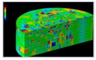
CASC's multiprocessor server allows to solve complex and node rich finite element simulations, such as a crystal plasticity simulation including soft and hard slip systems in MgO. Three dimensional crystal plasticity simulations are being carried out using parallel processing on the CASC cluster. It has been used to simulate the relation between primary and secondary slip
