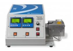
It is a three-part system: Extruder with Take Up, and Chopper Accessories. Maximum temperature 400°C and Variable speed control, 5 to 260rpm.
