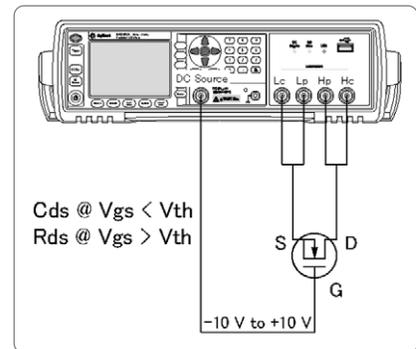
Figure 8. Measurement using DC source.
