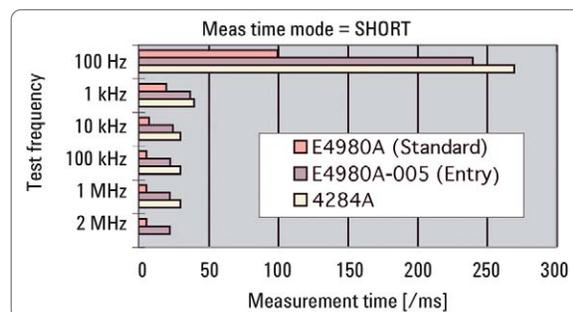
Figure 13. Measurement speed: standard E4980A LCR vs. economy model E5980A-005 LCR vs. 4284A LCR.
