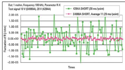
Figure 2. Low impedance evaluation (1 mΩ at 100 kHz).
