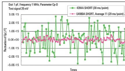
Figure 3. High impedance evaluation (1 pF at 1 MHz).
