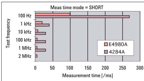
Figure 4. Measurement time<sup>1</sup>: standard E4980A LCR vs. 4284A LCR.
