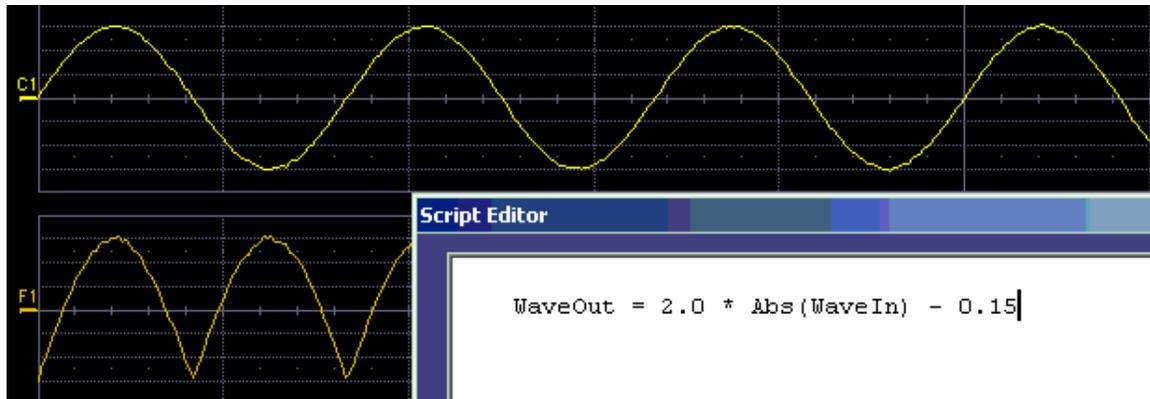
WaveOut is the waveform being returned to the instrument (F1 in this case). WaveIn is the input waveform (C1 in this case) You can see that the F1 result is displayed on the scope, and can be processed further.
