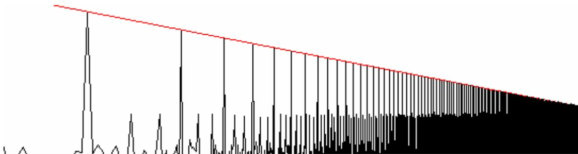
These examples were made with two different instrument setups: in the second, the FFT was zoomed vertically. The graph has a red line to represent the theoretical envelope for the peaks. This has great potential for testing the transmission characteristics of amplifiers and filters, since the output can be compared with a theoretical curve. Furthermore, if the output is divided by the
