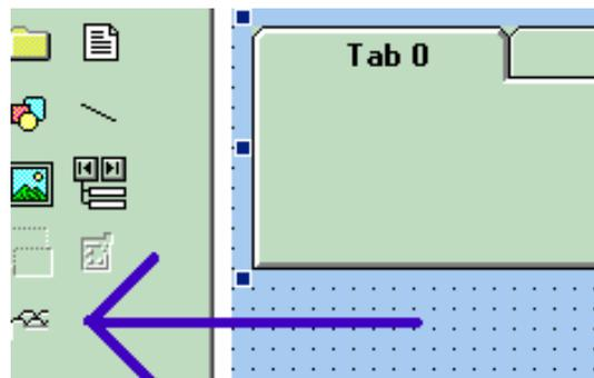
The system is very versatile, and you can place controls on the tabs of the Tabbed Control. Look in the properties window to see how you can customize your tabs, as illustrated below.
