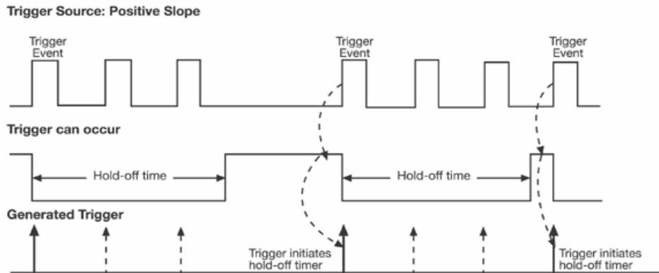
**Edge Trigger with Holdoff by Time.** The bold edges on the trigger source indicate that a positive slope has been selected. The broken upward-pointing arrows indicate potential triggers, which would occur if other conditions are met. The bold arrows indicate where the triggers actually occur when the holdoff time has been exceeded.
