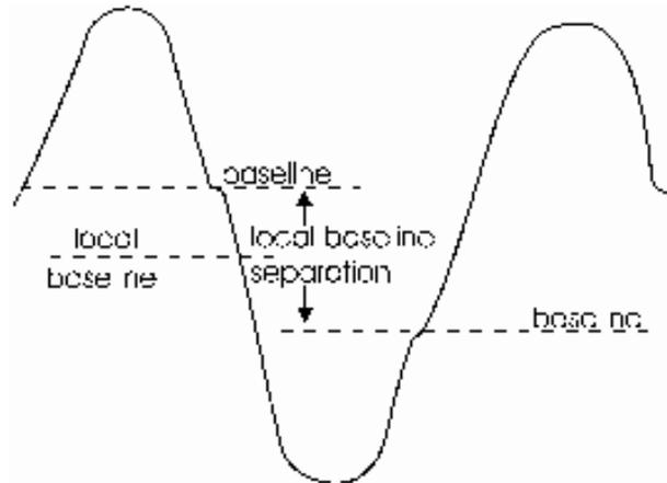
The baselines are found by locating a point at which the waveform 'rests' between the peak and trough and peak. These resting points are identified by statistically measuring the area of least change in voltage value between the peak and trough or trough and peak, with internal tolerance levels set to ensure against false baseline identification.
