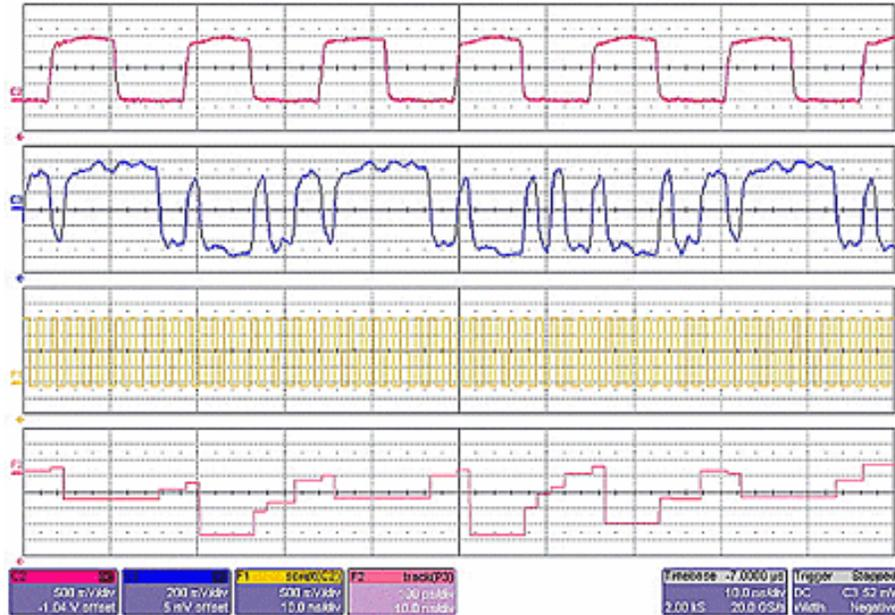
Example 4 is a measurement of DVI (Digital Video Interface) Data-Clock skew jitter measurement, using a VBScript to emulate the PLL.
