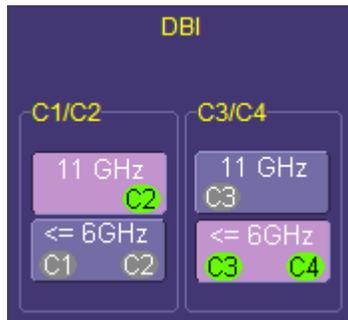
When 11 GHz is selected, the active channels are either C2 or C3 or both, providing 40 GS/s sampling on each channel. For 6 GHz bandwidth, all four channels can be used, providing 20 GS/s sampling on each channel. Channels can be set to allow 11 GHz and 6 GHz bandwidths at the same time, as shown at left.
