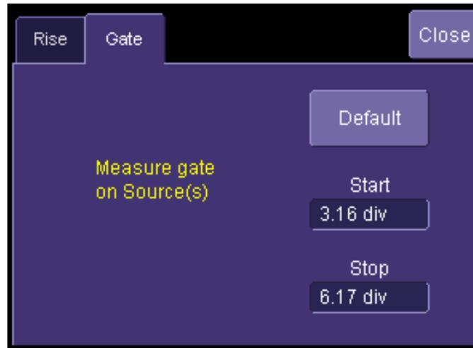
In this example, you can see that the Measure Gate includes only five rising edges. Therefore, parameter calculations for rise time are performed only on the five pulses bounded by the gate posts. The position of the gate posts is shown in the **Start** and **Stop** fields in the accompanying dialog.
