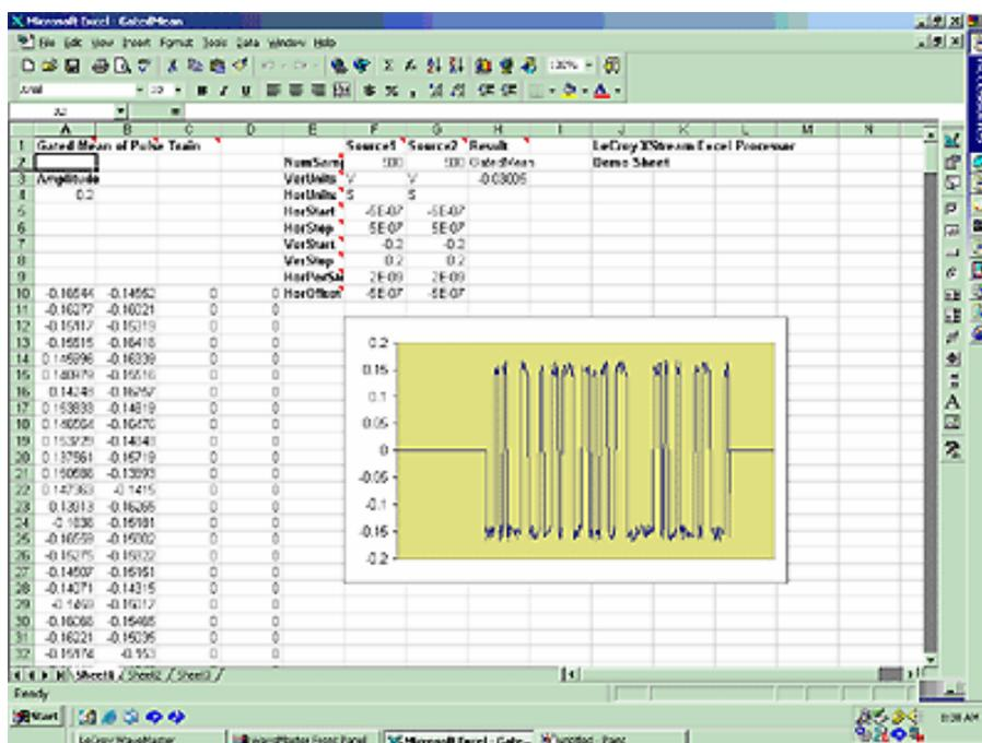
Here we see the gated waveform that has been created in Excel. The Mean parameter during the region of interest (ROI) is placed in cell H3.
