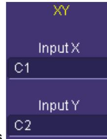
3. Touch inside the **Input X** and **Input Y** data entry fields and select your input sources from the pop-up menus. The inputs can be any combination of channels, math functions, and memory locations.
