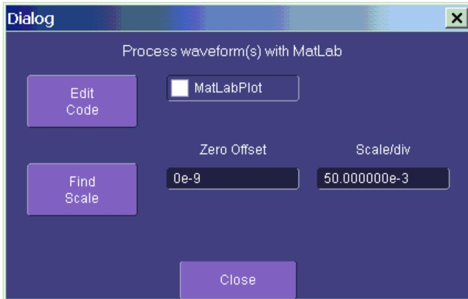
Touch **Find Scale** to make your output fit the grid, or use the text boxes to choose a scale.
