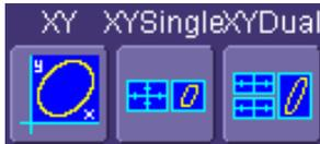
You have the choice of showing the two waveforms on just the XY grid, or you can also show the input waveforms on a single or dual grid.
