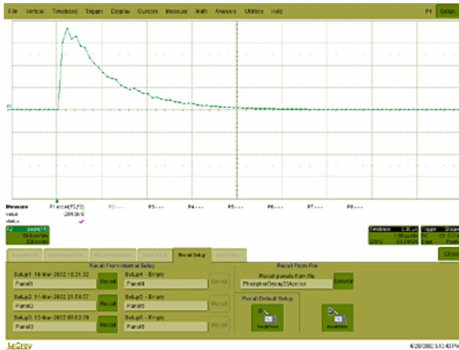
The pulse was generated by a formula of the form  $e^{-(1-t/TC1)} * e^{-t/TC2}$ , where TC1 and TC2 are time constants. The requirement is to measure the time constant TC2, using the portion of the trace where TC1 has negligible effect. This was done using Function F1, which is not a part of the measurement process.
