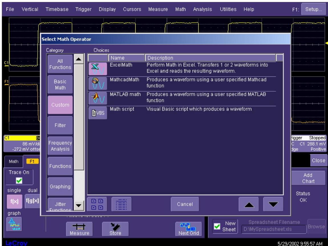
3. Choose File, Minimize from the menu bar to minimize the instrument display and open the Excel program.
