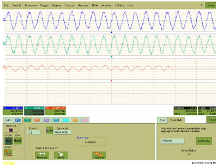
The noise was generated using pseudo-random numbers. Randomize Timer was included in the VBScript to ensure that the two traces differed, and that subsequent acquisitions differed. Functions F1 and F2 are included only to simulate signals, and are not part of the measurement process, which is performed by F3.
