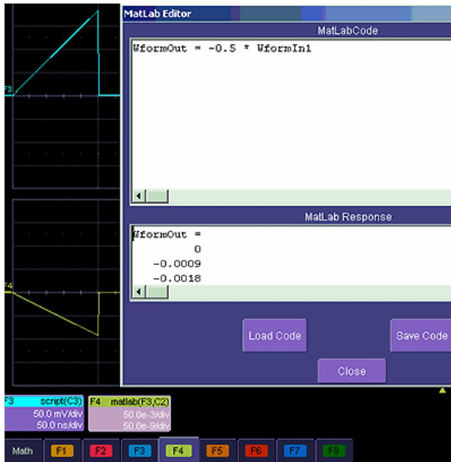
This is the default waveform function, with one important change: the semi-colon (;) has been removed from the end of the line. If the semicolon is present, your function will run much faster, because the output values will not be shown in MATLAB Response. With a long waveform, the time needed to display it could be quite long. The response values can be useful during development and debugging. Any line without a semicolon will produce a visible MATLAB Response.
