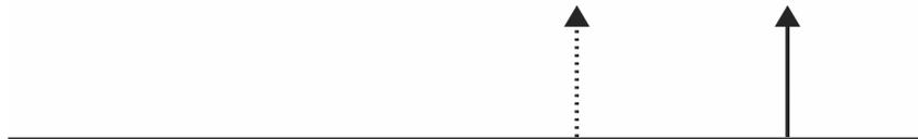
*Interval Trigger that triggers when the interval width is smaller than the selected interval. The broken, upward-pointing arrow indicates a potential trigger, while the bold one shows where the actual trigger occurs on the positive edge within the selected interval.*
