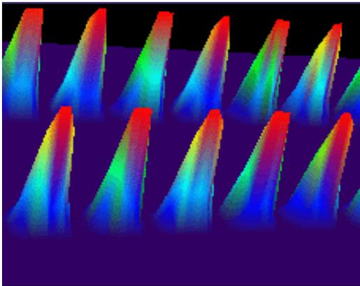
Here is an example of a 3-dimensional view of a square wave using the **solid** view of color-graded persistence. Saturation is set at 50%, with red areas indicating highest intensity. The X-axis has been rotated 60%; the Y-axis has been rotated 15%.
