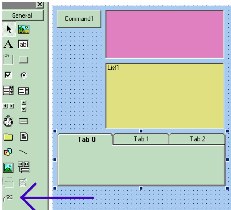
The Tabbed Control (arrow) is not in the basic tool box. To gain access to it, right click in the tool box at left (but not on an icon.) You will see this menu:
