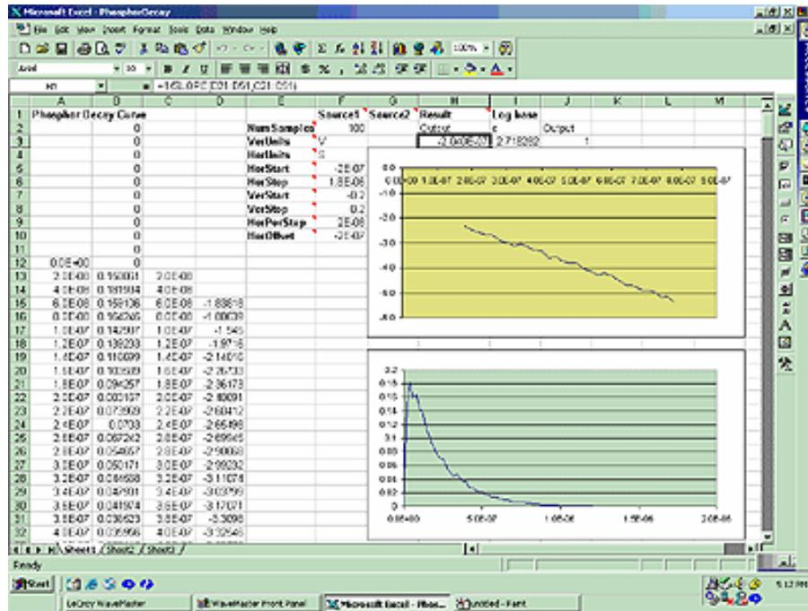
Here we see the input data in column B (with a time scale in A) created using the contents of cell F9, Horizontal Per Step. The logarithmic data are in column D, with the time scale repeated in C. The output appears in cell H3, using the formula `=1/SLOPE(D21:D51,C21:C51)`.
