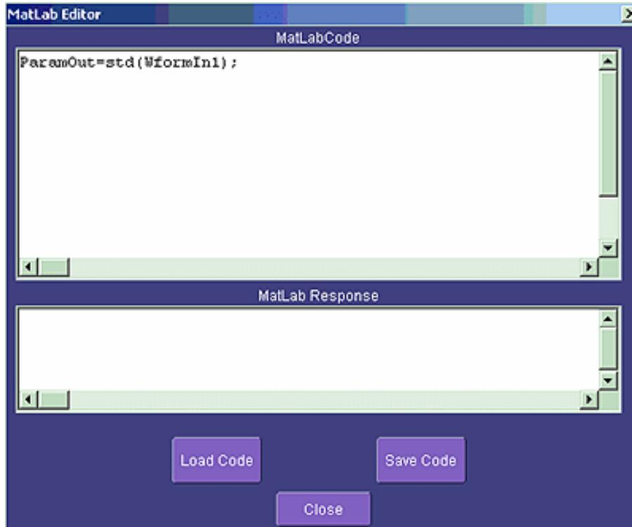
This simple example shows the MATLAB function Standard Deviation acting on input channel 1, and the result would be shown in the **MATLAB Response** pane for an amplitude of 0.15 volt.
