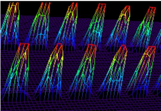
Here is a **wire frame** view of the same waveform in which lines of equal intensity are used to construct the persistence map.
