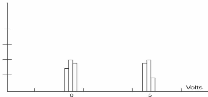
Determining such peaks is very useful because they indicate dominant values of a signal. However, signal noise and the use of a high number of bins relative to the number of parameter values acquired, can give a jagged and spiky histogram, making meaningful peaks hard to distinguish. The scope analyzes histogram data to identify peaks from background noise and histogram definition artifacts such as small gaps, which are due to very narrow bins.
