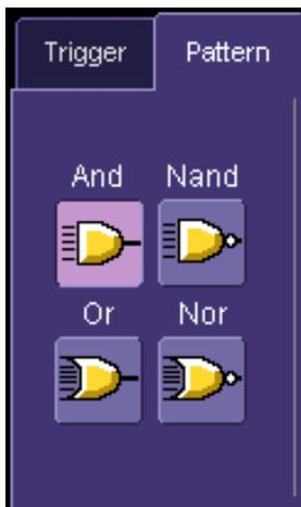
5. For each input you want to include in the logic pattern, touch inside the **State** field and select a logic state: Low or High. Select **Don't Care** for all other inputs.
