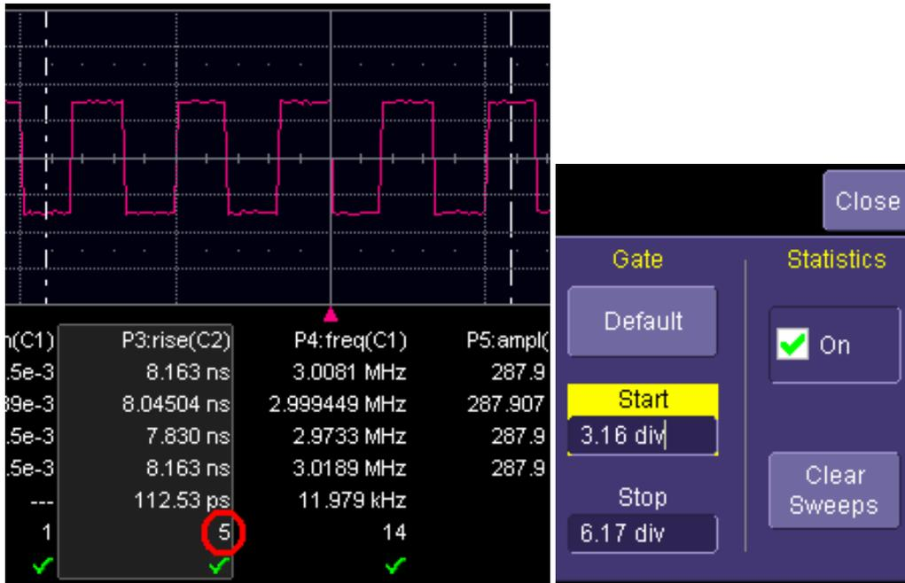
In this example, you can see that the Measure Gate includes only five rising edges. Therefore, parameter calculations for rise time are performed only on the five pulses bounded by the gate posts. The position of the gate posts is shown in the **Start** and **Stop** fields in the accompanying dialog.
