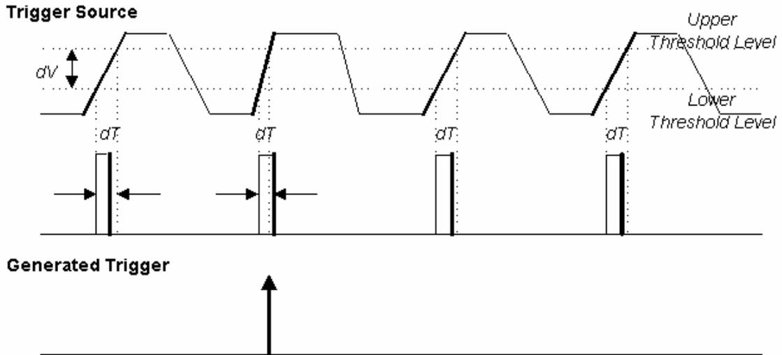
Slew Rate Trigger occurs when a rising or falling edge crosses two thresholds ( $dV$ ) outside a selected time range ( $dT$ ), indicated by the bold, upward pointing arrow.
