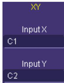
3. Touch inside the **Input X** and **Input Y** fields and select your input sources from the pop-up menus. The inputs can be any combination of channels, math functions, and memory locations.
