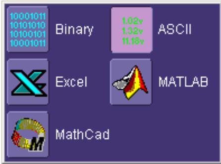
If you select **ASCII** or **Excel**, also touch the **SubFormat** field and select either **Time Data** or **Time & Ampl.** Then touch the **Delimiter** field and select a delimiter character from the pop-up menu: comma, space, semicolon, or tab.
