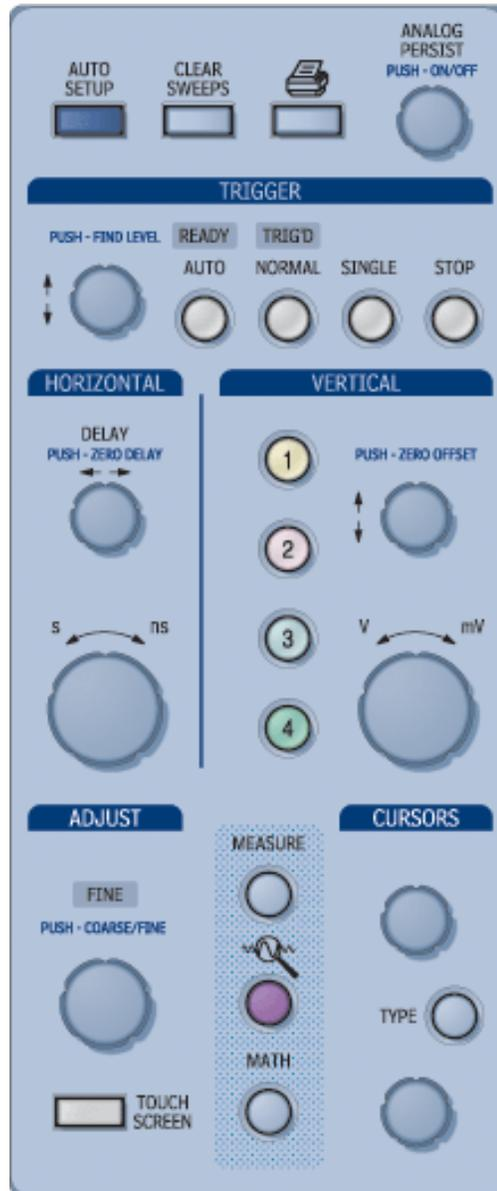
**Note:** Some of the front panel knobs are also special function push buttons. By pressing the knobs, you can activate functions such as Find Level, Zero Vertical Offset, and Zero Delay. The Adjust knob functions as a toggle between fine and coarse adjustment.
