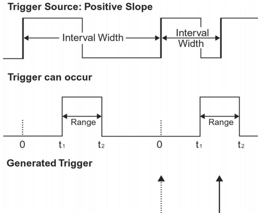
*Interval Trigger that triggers when the interval falls within the selected range:
