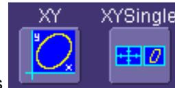
2. Choose an XY display by touching one of the XY display mode buttons. You have the choice of showing the two waveforms on just the XY grid, or you can also show the input waveforms on a single.
