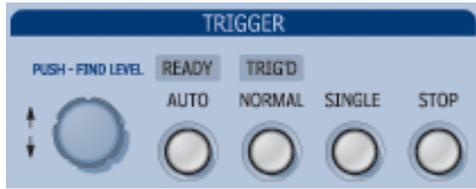
The *level* knob selects the trigger threshold level. Push this knob to quickly find the level, which is indicated in the **Trigger** descriptor label:
