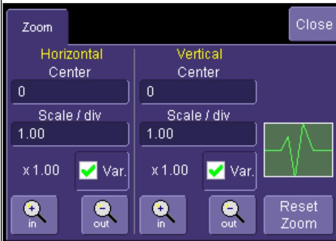
To unzoom a Memory or Math trace, push the front panel Horizontal **DELAY** and Vertical **OFFSET** knobs, which resets the trace to x1.00 magnification. Alternatively, touch the **Reset** button in the "Zoom" dialog.
