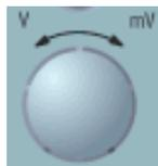
for the selected channel. Or you can touch inside the Volts/Div field in the channel setup dialog and type in a value using the pop-up keypad, or use the up/down arrows.
