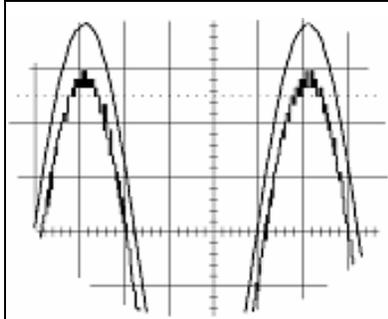
**To increase vertical resolution:** In the example at left, the lower ("inner") trace has been significantly enhanced by a three-bit enhanced resolution function.
