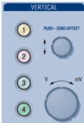
The Vertical Offset knob adjusts the vertical offset of a channel. Press the knobs to quickly set the offset to zero for the selected channel.
