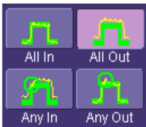
This selection means, for example, that if you select **All Out** the test will be False if even a single waveform falls inside the mask.
