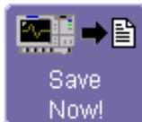
Then touch **Save Now!** below the data entry field. To save to folder **Internal Setup**s on the scope's hard drive, touch inside a **SetupX** data entry field and use the pop-up keyboard to enter a file name.
