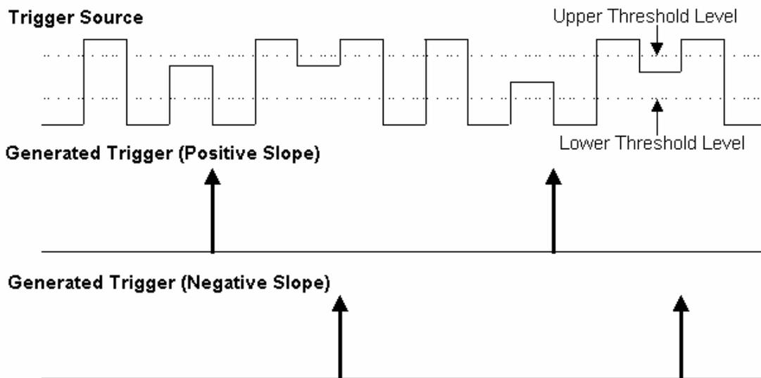
**Runt Trigger triggers when a pulse crosses the first threshold but not the second before recrossing the first (indicated by the bold, upward pointing arrows).**
