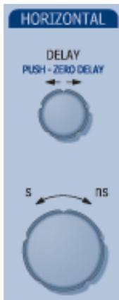
**DELAY** horizontally positions the scope trace on the display so you can observe the signal prior to the trigger time. It adjusts the pre- and post-trigger time. Push this knob to quickly set the delay to zero, in which case the trigger point is positioned in the middle of the display grid.
