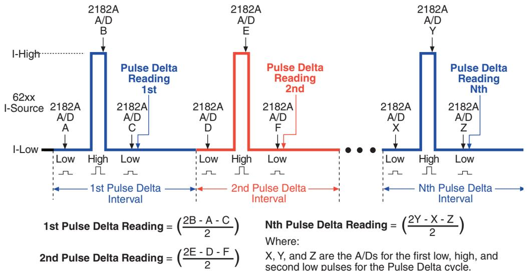
In cases where the high pulse will cause heating of the Device Under Test (DUT), the measurement at the second low pulse could be adversely affected by the heat caused by the high pulse. In that case, the measurement at the second low pulse can be disabled. This does not change the overall timing of the pulse output. Eliminating the second low pulse measurement changes the basic calculation to the following:
