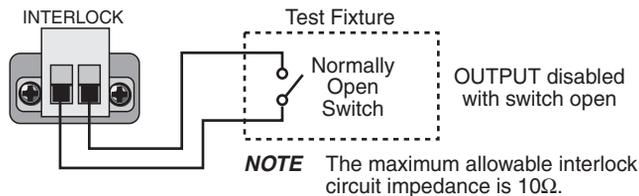
**WARNING** An open INTERLOCK only disables the output from the Model 622x. If an external source is being used in the test circuit, its voltage will be present in the test circuit. A hazardous voltage from an external source could be connected directly to the OUTPUT connector of the Model 622x.
