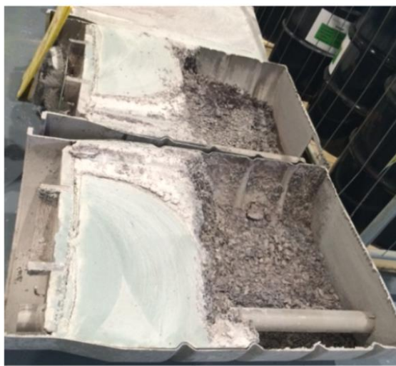
Below: Waste immobilisation through cement encapsulation at Workington
