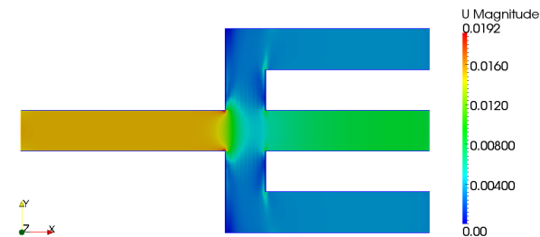
Figure 7.31: Triple outlet duct manifold velocity contour plot for case B = 1\text{T} , Ha = 108 , t_w = 0.01 . Manifold region insulating, outlet ducts conducting with EM coupling.
