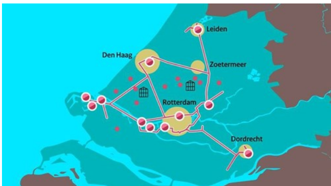
The heat roundabout in Rotterdam, industry supply heat to municipal heat networks and greenhouses.
