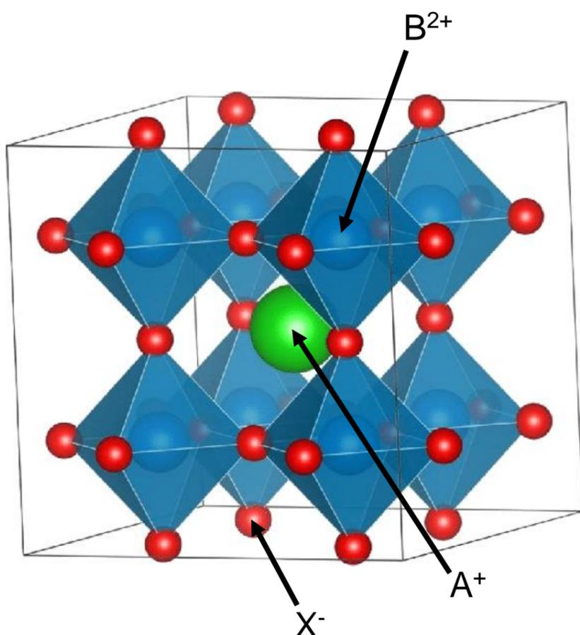
The perovskite crystal structure<sup>1</sup>.
