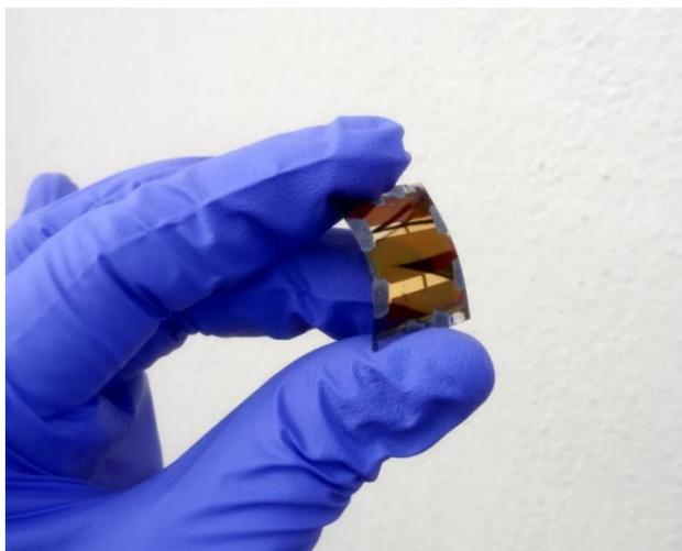
A flexible perovskite solar cell module<sup>3</sup>.
