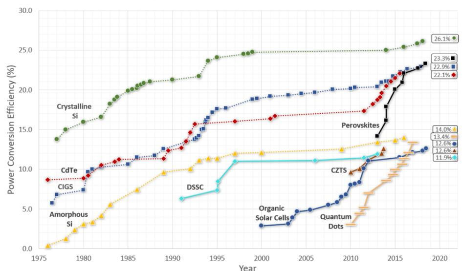
This graph shows the increase in solar cell efficiency with time for a variety of technologies<sup>4</sup>.
