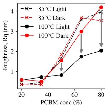
*In-situ* NR from 20 – 100 °C, with and without light: Measurements of Si/PEDOT:PSS/PS:PCBM while annealing to monitor changes perpendicular to the substrate.
