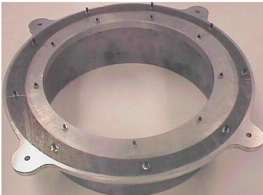
Figure 5.6: stator mount
