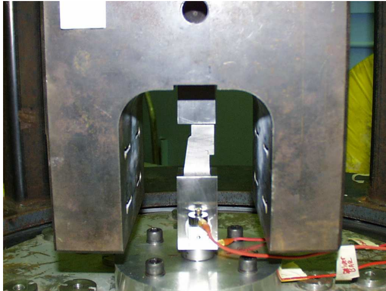
Figure 4.62. Experimental Setup of the Solid, Stainless Steel Leg.
