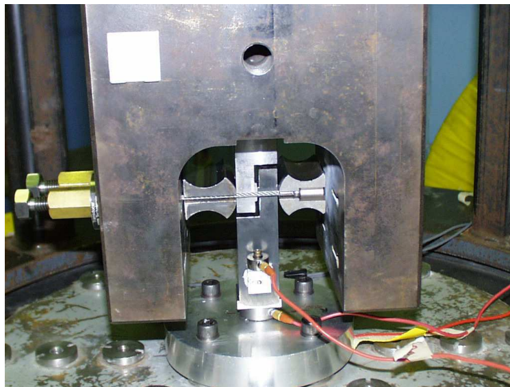
Figure 4.12. Stepped Specimen Setup.
