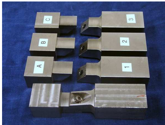
Figure 5.50. AOS Single-Leg Specimens.
