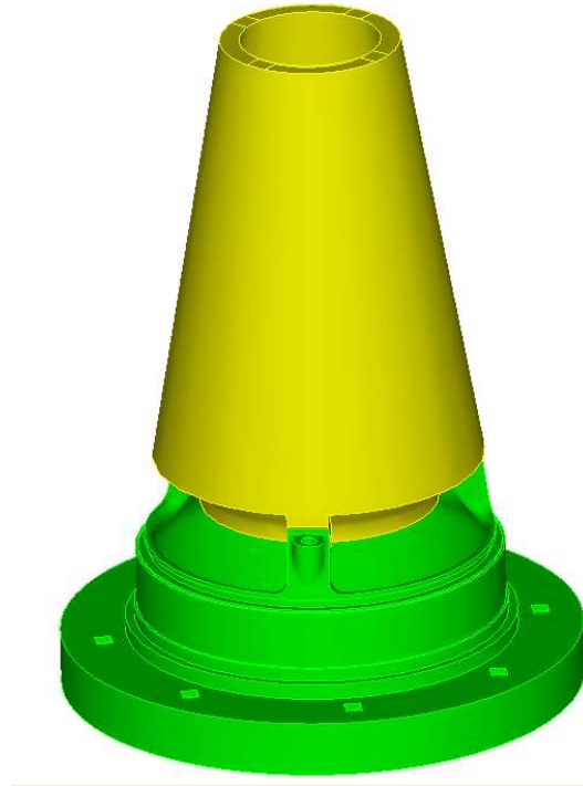
Figure 18.4. Solid Geometry Representation of a Forward Mount/Mass Mock.
