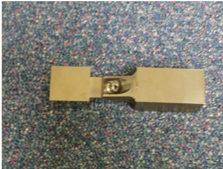
Figure 4.56. AOS Single-Leg Test Specimen with a Bolt.
