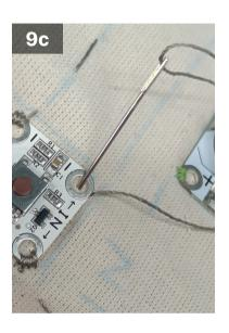
Bring the needle down through the fabric into the negative 'in' hole.
