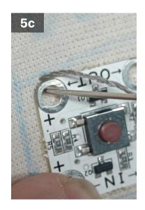
Bring the needle down into the positive 'out' hole to sew a tight stitch.
