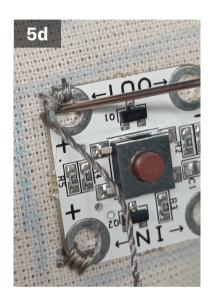
Sew 4 more tight loops around the positive out hole in the switch module.
