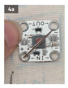
Hold the switch down with the 'in' side facing the cell holder.
