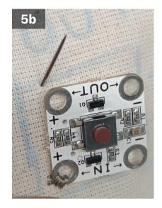
Bring your needle up through the fabric **near** the **positive hole** of the switch on the **'out' side**.
