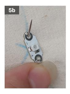
Insert your needle from the back side of the fabric, coming up through the **negative terminal of the LED**.
