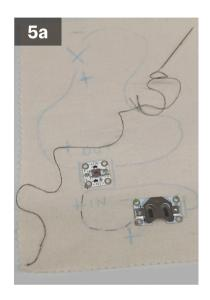
Re-thread your needle with **conductive thread**.
