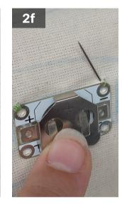
Check coin cell holder for **positive** and **negative** markings.
