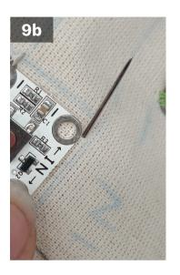
Bring your needle up through the fabric near the **negative hole of the switch on the 'in' side.**
