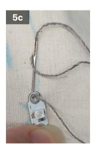
Stitch **5 tight loops** around the negative terminal building a secure connection.
