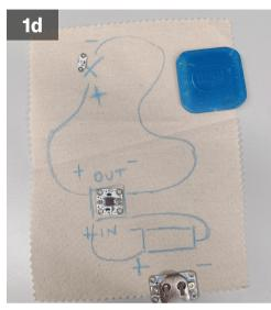
Draw a line connecting the + 'out' hole of the switch to one side of the LED. Mark that LED side with a + sign.
