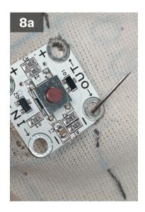
Bring your needle up from the back of the fabric into the **negative hole** on the **'out' side** of the switch.
