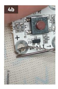
Bring the needle back down outside of the hole to sew a **tight loop around the edge.**
