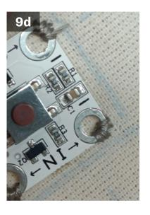
Sew 4 more tight loops around the negative in hole in the switch module.
