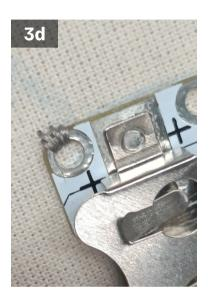
Stitch 4 more loops close together around the circular hole. You should build up a thick thread connection to the metal.
