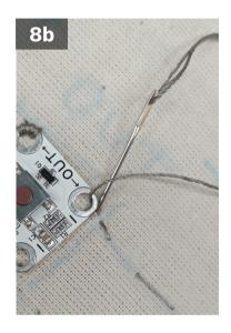
Bring the needle back down through the fabric outside of the hole to sew a **tight loop around the edge.**
