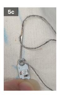
Stitch **5 tight loops** around the negative terminal building a secure connection.
