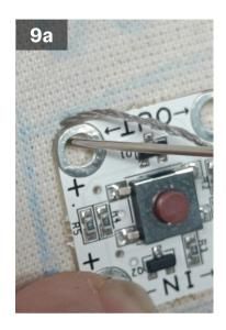
Rethread your needle with a new length of conductive thread.
