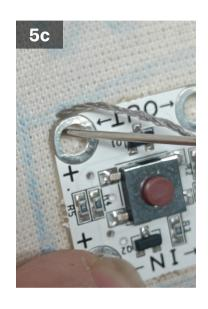
Bring the needle down into the positive 'out' hole to sew a tight stitch.
