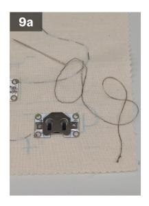
Re-thread your needle with conductive thread.
