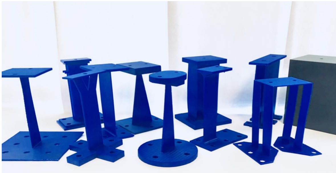
Figure 3. Various designs were produced and manufactured including column piers, frames, and shell structures. (Note: Holes in the base are for clamping purposes).
