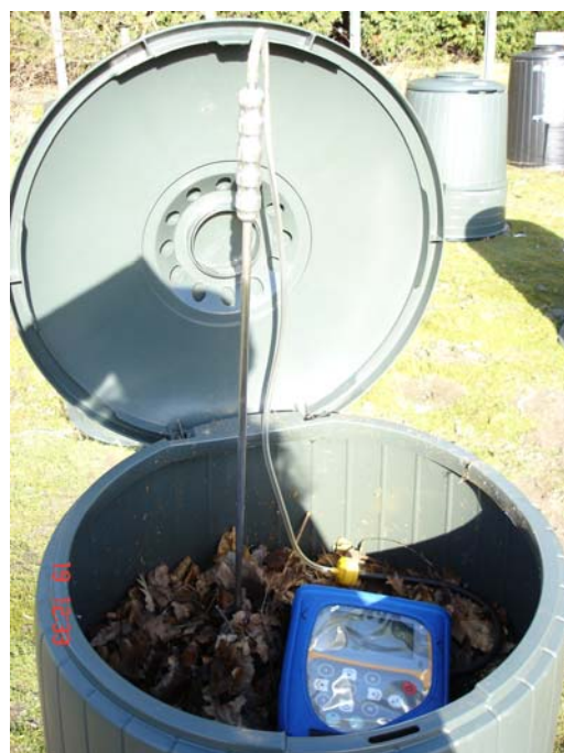
Figure 2.12 Monitoring interstitial gases with portable equipment
