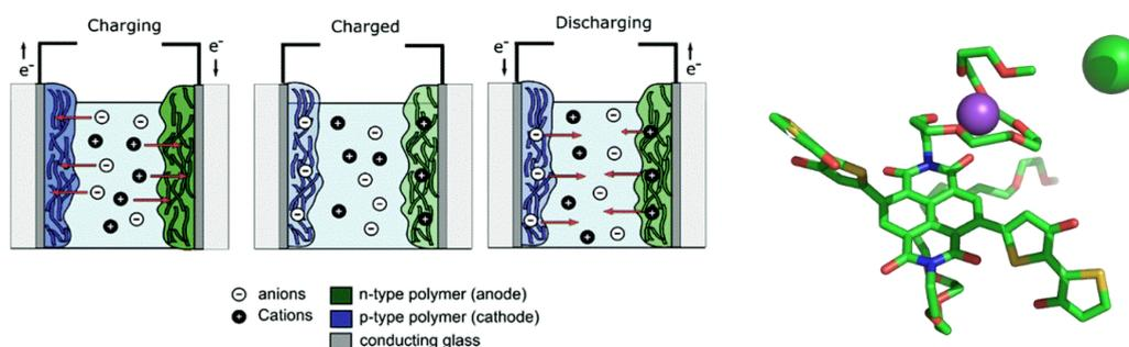
**Figure 1:** Left: schematic of the polymer battery concept; Right: molecular dynamics snapshot of ion-polymer interaction.
