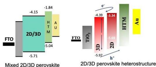
Figure 1. Schematic illustration of the dimensionally engineered 2D/3D perovskite thin film bandgap diagrams in mixed and heterostructure devices.
