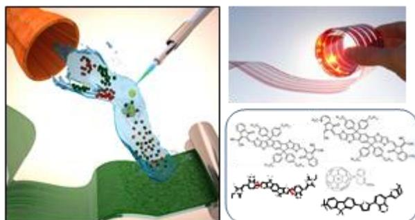
Schematics of printing flexible OPV devices (left), printed flexible OPV modules (top right), organic electron acceptors including NFAs (bottom right)
