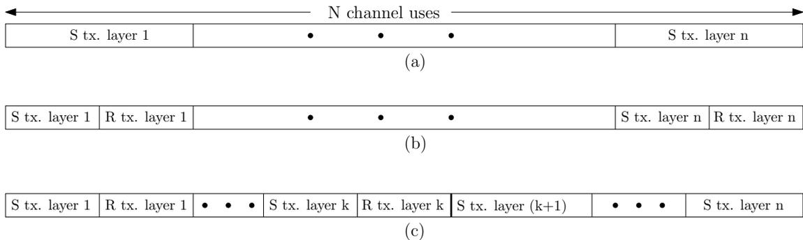
Fig. 6. Illustration of LS strategy with (a) only direct transmission, (b) only simple cooperative relaying, and (c) with both cooperative relaying and direct transmission.
