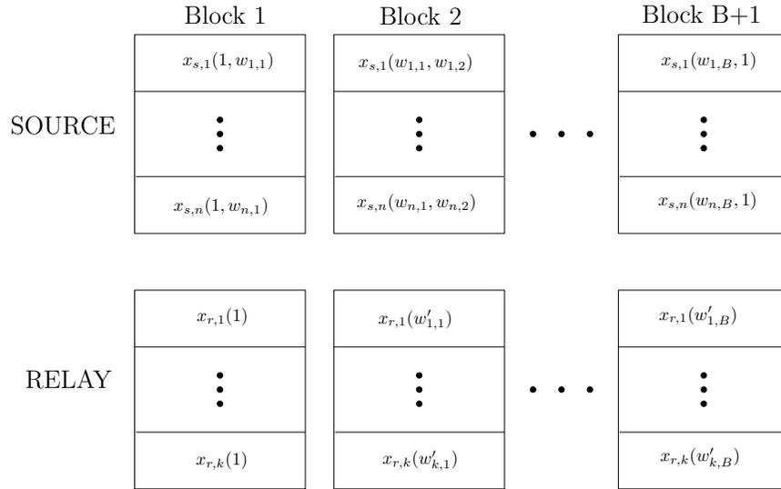
Fig. 12. Block Markov encoding for full duplex relay BS. In the figure, it is assumed that the relay can decode, and thus can forward, up to layer  $k$ . Also  $w'_{b,j}$  denotes the relay's estimate of layer  $j$  in block  $b$ .
