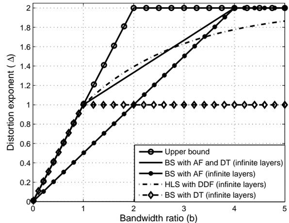
Fig. 10. Distortion exponent vs. bandwidth ratio of BS strategy using different cooperative protocols. For comparison, the full-duplex upper bound, and HLS with DDF are also shown.
