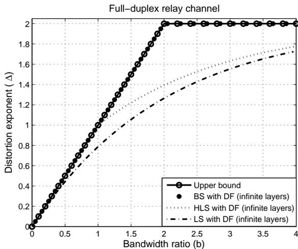
Fig. 11. Distortion exponent vs. bandwidth ratio for the full-duplex cooperative relay channel.
