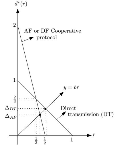
Fig. 2. A geometric interpretation illustrating the optimal multiplexing gain and distortion exponent for a single layer source-channel coding system.
