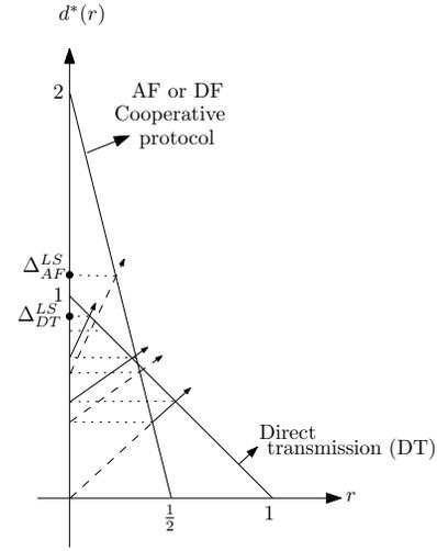
Fig. 5. A geometric interpretation of the LS strategy in the case of multiple source layers. Straight lines climb the DT curve, while the dashed ones climb the cooperation curve.
