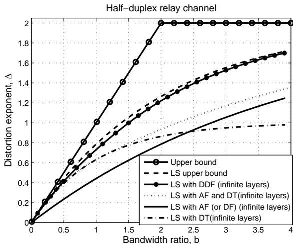
Fig. 7. Distortion exponent vs. bandwidth ratio for LS using different cooperation protocols.
