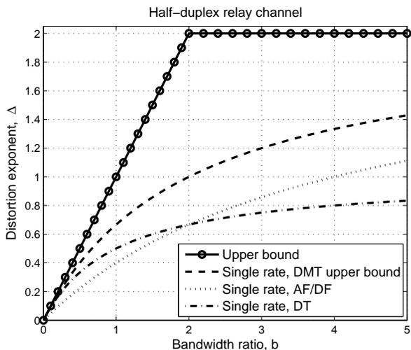
Fig. 3. Distortion exponent of single rate transmission with direct transmission and simple AF/DF cooperation.
