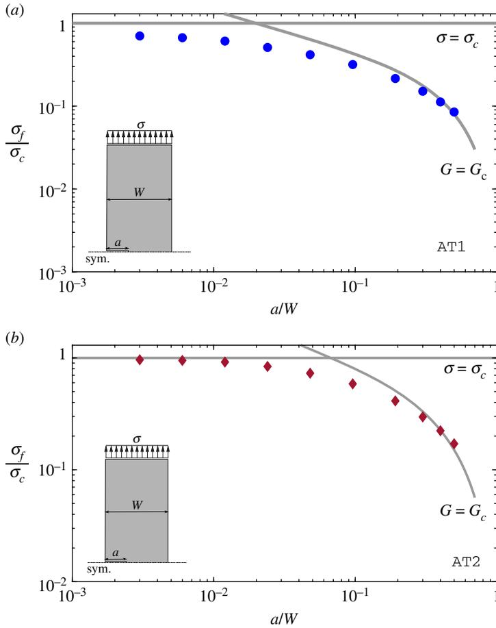
**Figure 12.** Transition flaw size analysis: failure strength as a function of the crack size for (a) AT1, and (b) AT2 phase field models. The solid grey lines denote the fracture predictions according to the material strength and to Griffith's criterion (4.10). (Online version in colour.)
