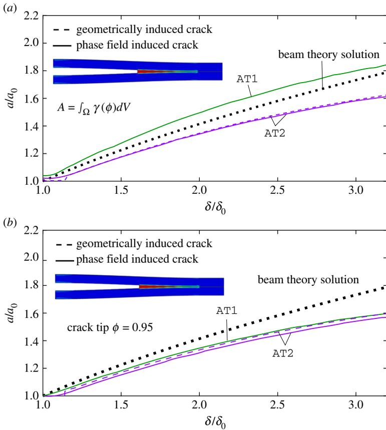
**Figure 10.** Double cantilever beam analysis. Crack extension as measured by: (a) the crack surface density function, equation (2.12), and (b) the furthest point with  $\phi = 0.95$ . (Online version in colour.)
