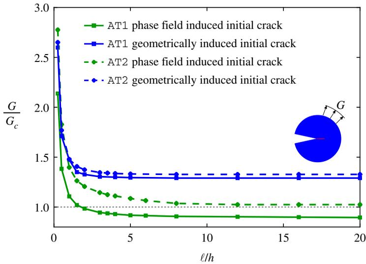
**Figure 4.** Boundary layer analysis: Mesh sensitivity of the energy release rate at initiation of crack growth for different constitutive choices and approaches for implementing the initial crack. The value of the characteristic fracture length scale to the phase field length scale is  $L_f/\ell = 10$ . (Online version in colour.)
