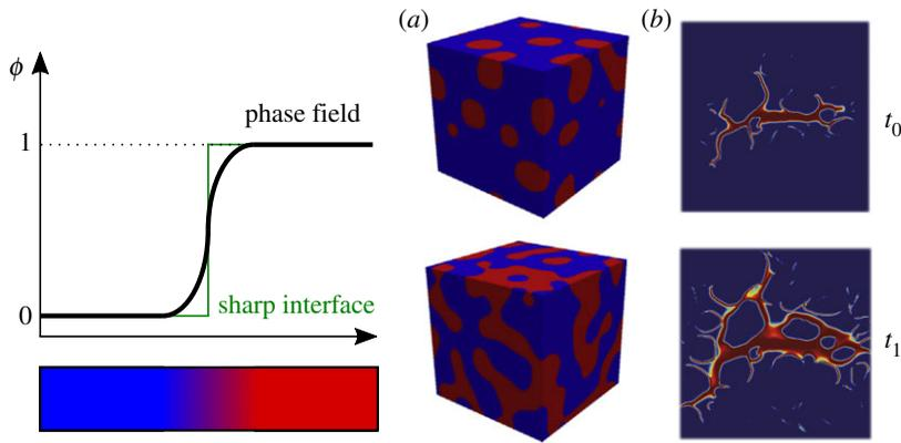
**Figure 1.** Tracking interfaces *implicitly* using an auxiliary phase field  $\phi$ . Examples capturing (a) microstructural evolution [32], and (b) the propagation of cracks [33], for two instants in time ( $t_0, t_1$ ). (Online version in colour.)
