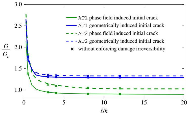
**Figure 6.** Boundary layer analysis: influence of enforcing damage irreversibility on the initiation of crack growth. Symbols denote the results without the irreversibility condition, equation (3.3). The value of the characteristic fracture length scale to the phase field length scale is  $L_f/\ell = 10$ . (Online version in colour.)
