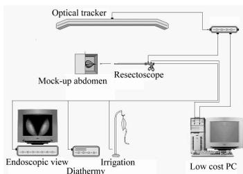
In CASTS (left), the trainee resects a prostate phantom, inserted in a mock-up abdomen, using standard real surgical tools, instrumented for optical tracking (right). A GUI displays a model of the phantom, the position of the resectoscope and the tissue resected.
