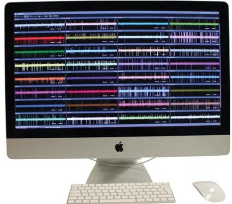
Software platform for configuration and real-time visualization of neural recording and spike sorting.
