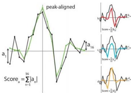
Distance based template matching method. Colour traces are templates. Black traces are input signals. The score is the sum of distances between signals and templates. The matching template achieves the lowest score that is below a user set threshold.
