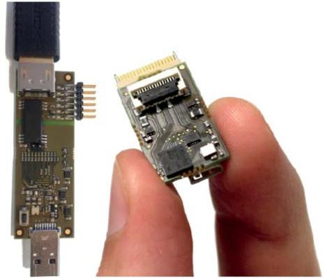
NGNI V1 platform showing 32-channel headstage and USB3.0 SS bridge.
