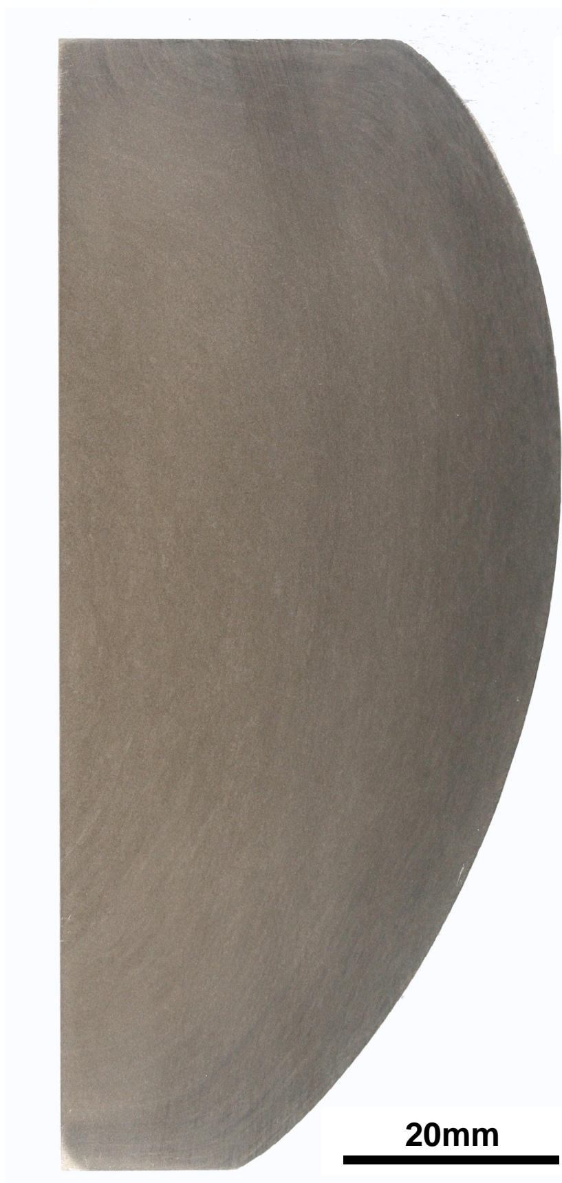
Figure B 5. Photograph of forged Ti-6Al-4V segment D2, etched to reveal the forging flow lines.
