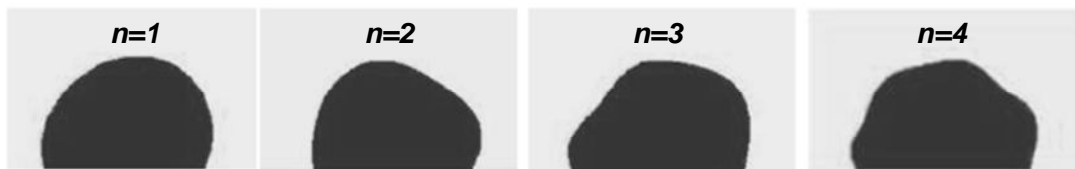
Figure 19. Simulated first four modes of vibration of a water droplet. After Dong et al [51].
