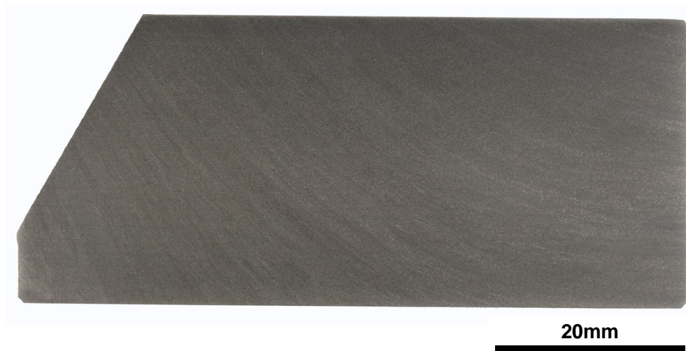
Figure B 17. Photograph of forged Ti-6Al-4V segment N, etched to reveal the forging flow lines.
