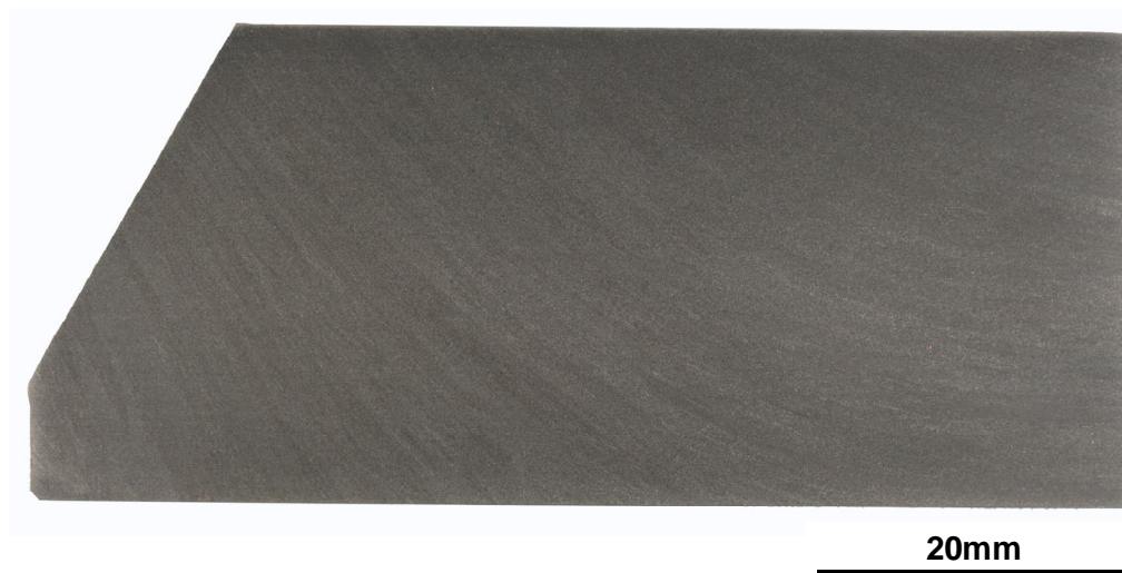
Figure 32. Photograph of forged Ti-6Al-4V segment N, swab etched with 10% HF, 50% HNO 3 in water to reveal the forging flow lines.
