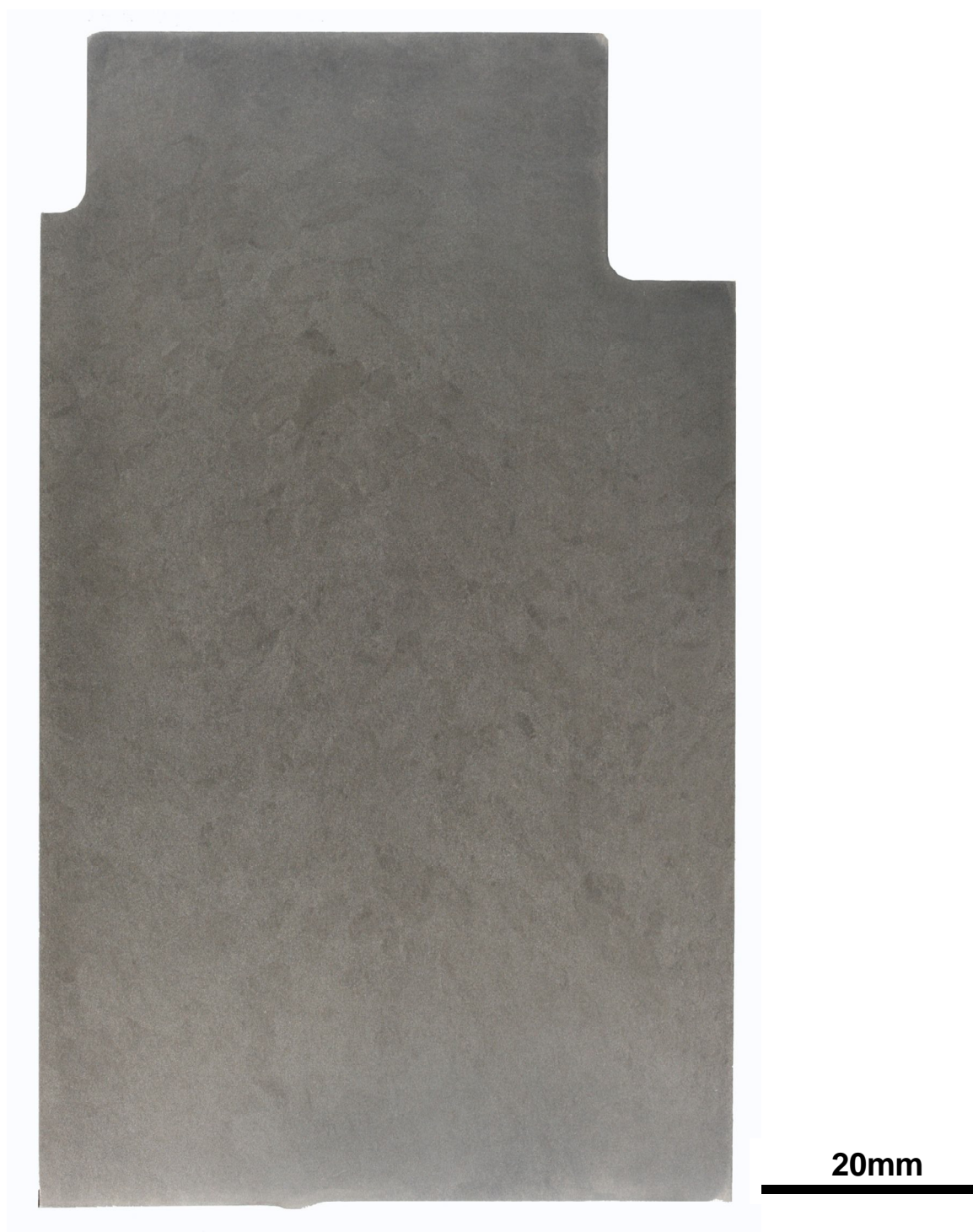
Figure B 9. Photograph of forged Ti-6Al-4V segment J, etched to reveal the forging flow lines.
