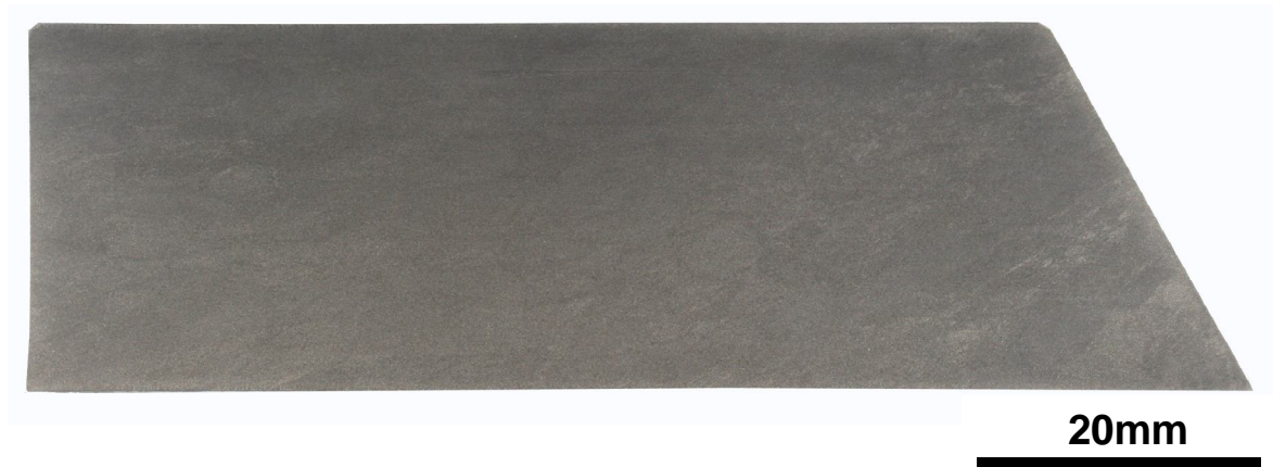
Figure B 13. Photograph of forged Ti-6Al-4V segment M, etched to reveal the forging flow lines.
