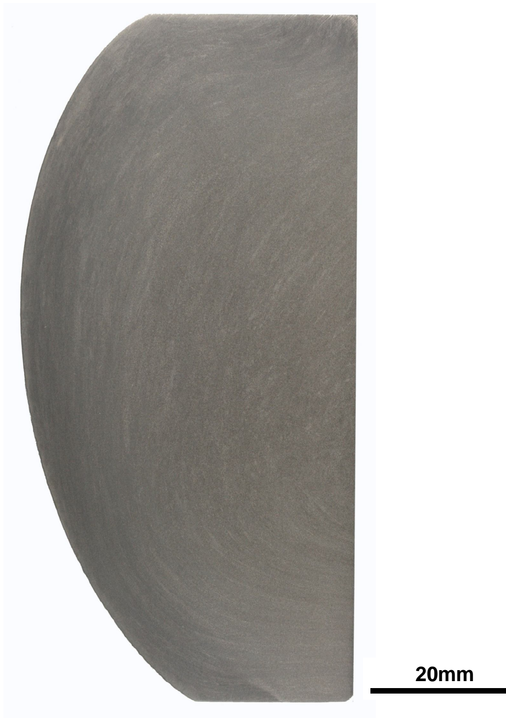
Figure B 1. Photograph of forged Ti-6Al-4V segment D1, etched to reveal the forging flow lines.
