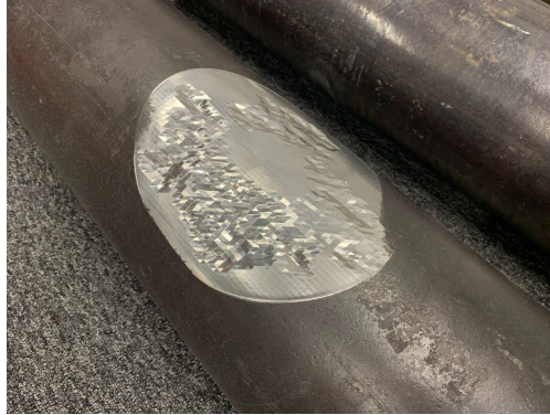
Figure 3.17: Artificial corrosion patch manufactured on Pipe 2, which has a radius of approximately 80 mm and a depth of 5.32 mm, representing a 40% loss in thickness.
