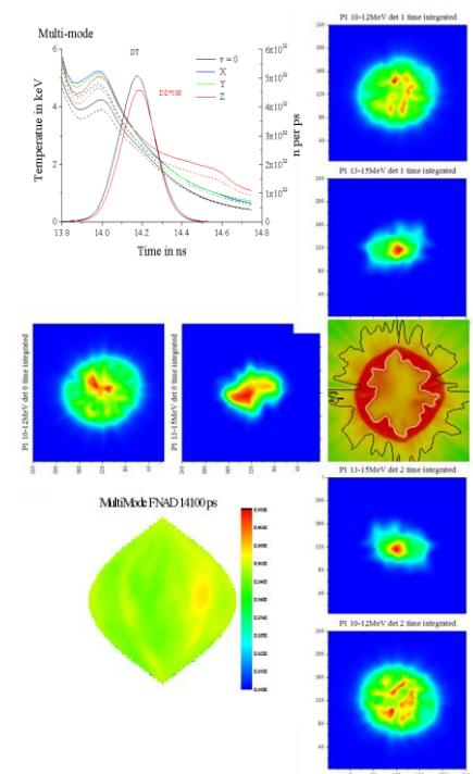
time. These show that whilst the inferred temperatures are fairly isotropic the temperature inferred from DT spectra are consistently higher than those from DD spectra (by about 300eV). This result is similar to that observed in experiment and is consistent with a hotspot with a finite but isotropic velocity variance<sup>5</sup>.
