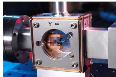
Single ion trap in  $^{171}\text{Yb}^+$  clock at NPL
