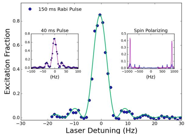
**Figure 1.** Coherent Rabi spectroscopy of the Sr clock transition for 40 ms (inset-left) and 150 ms (main)  $\pi$ -pulse, and spectroscopy of  $m_F$  states with and without spin-polarising (inset right).
