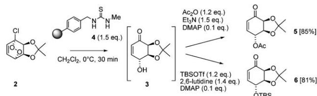
**Scheme 3** Sequential hydrogenolysis/protection of endoperoxide **2**.
