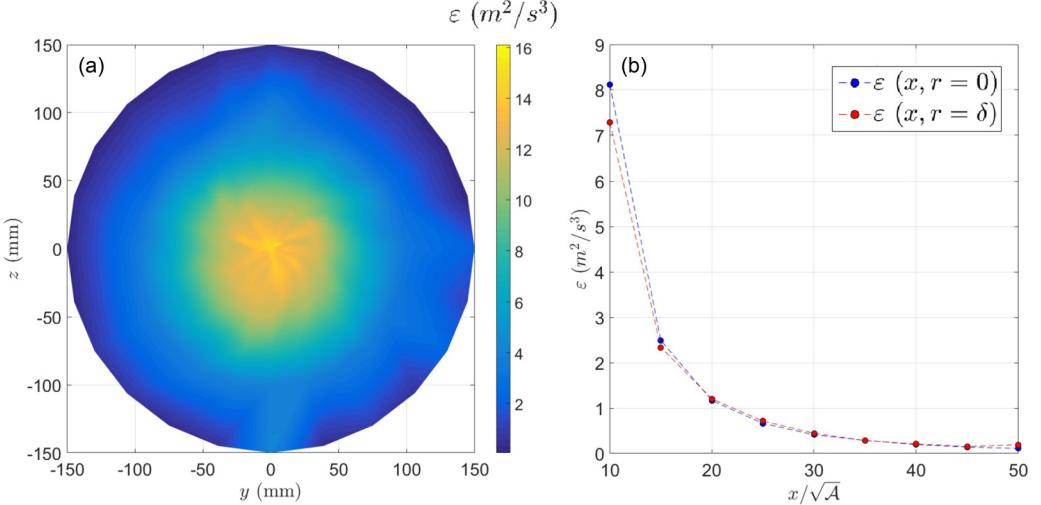
FIG. 4. Cross section of  $\varepsilon$  at  $x/L_b = 10$  (a). Comparison of the streamwise evolution of  $\varepsilon$  at  $r = 0$  (blue line) and  $r = \delta$  (red line) (b).  $\varepsilon$  was estimated using the same method as in Fig. 3.
