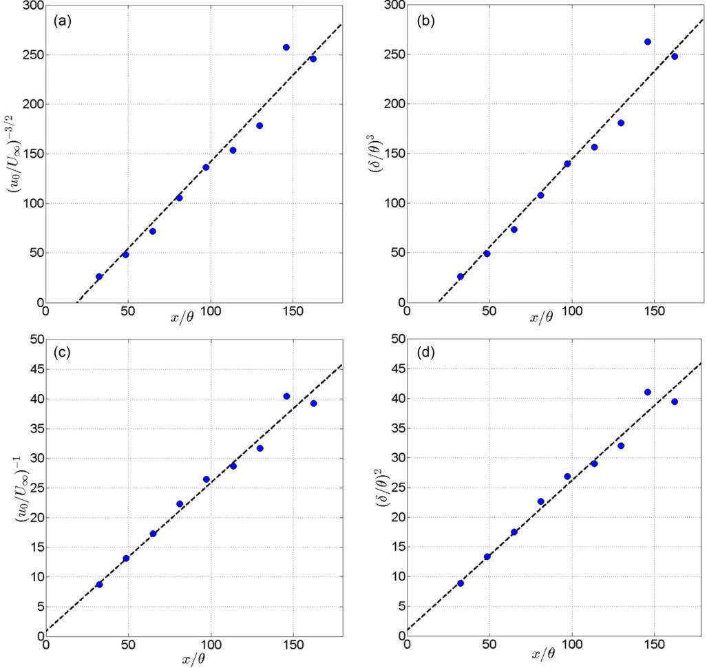
FIG. 5. Normalized velocity deficit linearized according to equilibrium scalings,  $(u_0/U_\infty)^{-3/2}$ , as a function of  $x/\theta$  (a). Normalized wake width linearized according to equilibrium scalings,  $(\delta/\theta)^3$ , as a function of  $x/\theta$  (b). Same parameters linearized according to nonequilibrium scalings:  $(u_0/U_\infty)^{-1}$  for the normalized velocity deficit (c) and  $(\delta/\theta)^2$  for the normalized wake width (d).
