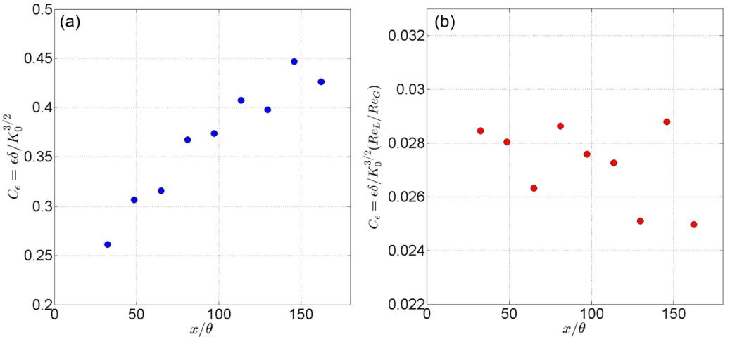
FIG. 3. Equilibrium dissipation coefficient  $C_\epsilon^{\text{Eq}} = \epsilon_0\delta/K_0^{3/2}$  (a). Nonequilibrium dissipation coefficient  $C_\epsilon^{\text{Noneq}} = \epsilon_0\delta/K_0^{3/2}(Re_L/Re_G)$  (b).
