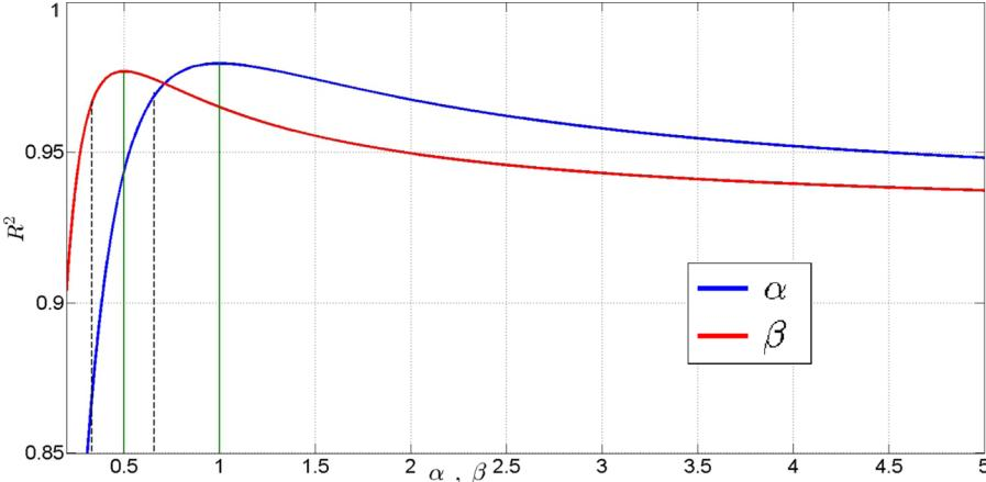
FIG. 6. Linear regression coefficient  $R^2$  as function of scaling exponents for  $u_0/U_\infty$  (blue line) and  $\delta/\theta$  (red line). The black vertical dotted lines locate the equilibrium scaling exponents while the green vertical lines locate the nonequilibrium ones.
