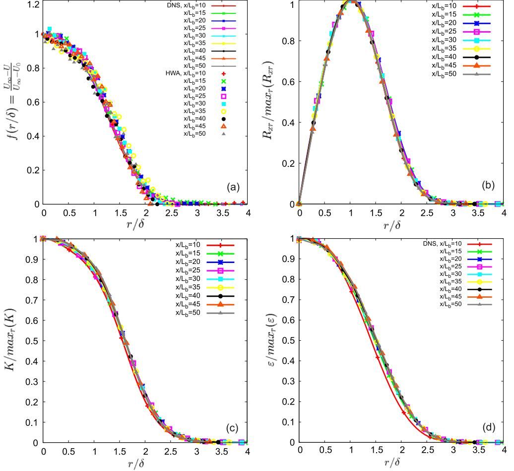
FIG. 1. Mean flow profiles at different streamwise distances plotted using similarity scalings (a). Markers stand for HWA measurements while lines stand for DNS data. Profiles of  $R_{xr}$  (b),  $K$  (c), and  $\varepsilon$  (d) normalized by the maximum radial value at different streamwise distances versus  $r/\delta$  for DNS only.
