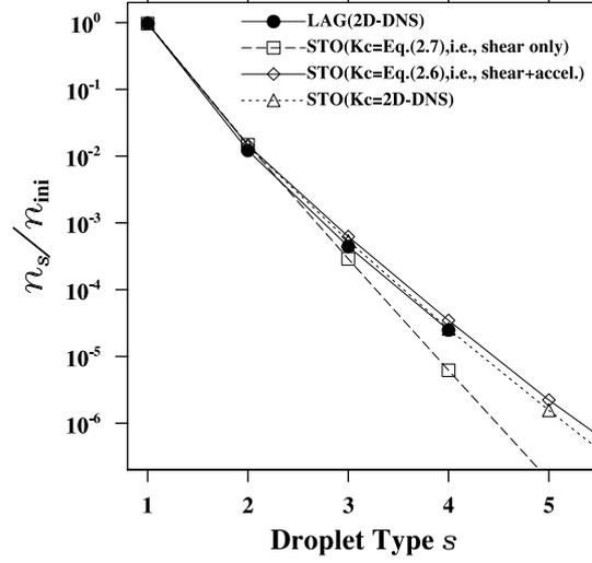
FIGURE 6. Distribution of droplet sizes produced from an initially uniform population at  $t/\tau_L = 9.5$ . LAG(2D-DNS) refers to the result obtained from a Lagrangian procedure applied to our 2D DNS, STO( $K_c$ =Eq.(2.7), i.e. shear only), STO( $K_c$ =Eq.(2.6), i.e., shear+accel.) and STO( $K_c$ =2D-DNS) refer to results obtained by solving the stochastic equation (4.2) with three different ways of obtaining collision kernels.
