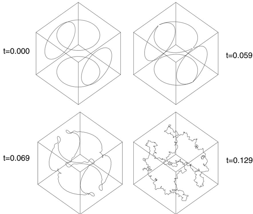
FIG. 1. Vortex configurations at  $t = 0.0$  sec (initial state, 576 points used; the vortex rings have a radius of 0.023 cm and the cube has size of 0.0639 cm),  $t = 0.059$  sec (first reconnection),  $t = 0.69$  sec (note the Kelvin waves), and  $t = 0.129$  sec (927 points used; note the crinkled shape of the filaments).
