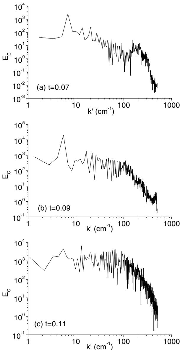
FIG. 3. Curvature spectra  $E_C(k')$ . (a)  $t = 0.069$  sec; (b)  $t = 0.089$  sec; (c)  $t = 0.109$  sec.
