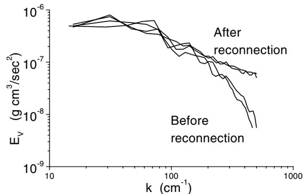
FIG. 2. Velocity spectra  $E_V(k)$  before the reconnections (lower two curves at  $t = 0.0$  sec and  $t = 0.030$  sec) and after the reconnections (upper two curves at  $t = 0.069$  sec and  $t = 0.089$  sec). The spectra are obtained by discretizing the computational box into  $64^3$  mesh points.
