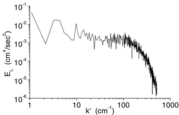
FIG. 5. Lagrangian velocity spectrum  $E_L(k')$  at  $t = 0.109$  sec.
