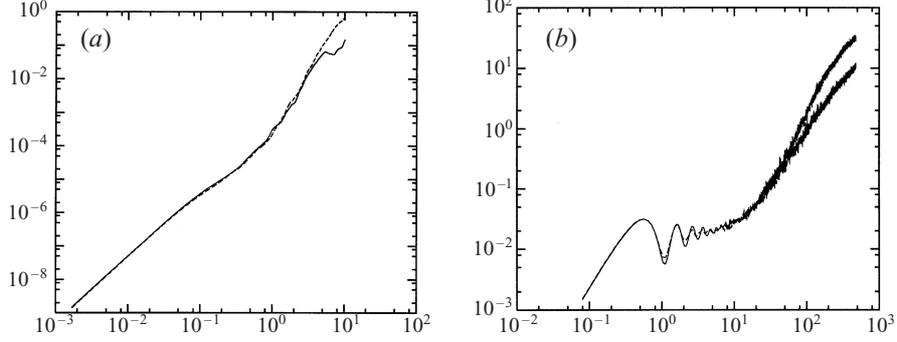
FIGURE 11. Two-particle turbulent diffusion obtained for  $Fr = 0.0034$  and  $Lk_{max} = 47$ , for steady case  $\lambda = 0$  (continuous line) and unsteady case  $\lambda = 1$  (dashed line). (a)  $\langle \Delta x_1^2 \rangle / L^2$  as a function of  $\tau u' / L$ , (b)  $\langle \Delta x_3^2 \rangle N^2 / (u' \Delta_0^2)$  as a function of  $\tau N / 2\pi$ .
