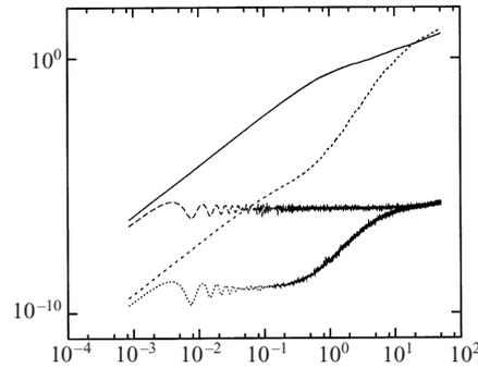
FIGURE 17. One- and two-particle diffusion,  $Fr = 0.0011$  ( $Fr_\eta = 0.02$ ),  $Lk_{max} = 47$  and  $\Delta_0 k_{max} = 0.2$ . Solid line:  $\langle x_1^2 \rangle / L^2$ , long dashed line:  $\langle x_3^2 \rangle / L^2$ , short dashed line:  $\langle \Delta x_1^2 \rangle / L^2$ , dotted line:  $\langle \Delta x_3^2 \rangle / L^2$ ; normalized time is  $\tau u' / L$ .
