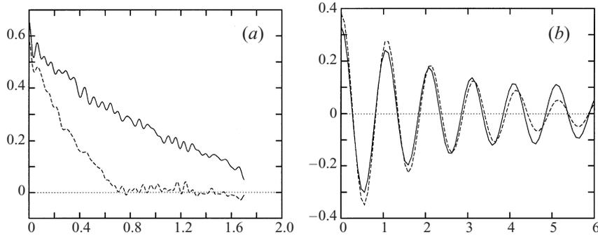
FIGURE 4. Non-dimensionalized KS Lagrangian velocity correlations for the same case as in figure 3. (a) Horizontal velocity correlation  $\langle u_{L1}(t_0)u_{L1}(t_0 + t)/u^2 \rangle$  as a function of non-dimensionalized time  $(t - t_0)u'/L$ . (b) Vertical velocity correlation  $\langle u_{L3}(t_0)u_{L3}(t_0 + t)/u^2 \rangle$  as a function of non-dimensionalized time  $(t - t_0)N/2\pi$ . Continuous line:  $\lambda = 0$ , dashed line:  $\lambda = 1$ .
