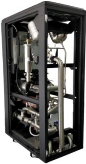
FS600 (DN65 hygienic flange connections)
