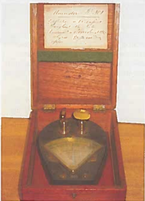
An ammeter, made in 1883 and designed to measure the flow of electric current, has its roots at Imperial
